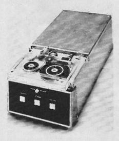
The tape drive on Model 330 is fully bi-directional at 25 ips normal speed, resulting in a data transfer rate of 40,000 bits/ second at 1600 cpi recording density it is claimed. Forward and reverse search modes, as well as rewind speed, are 90 ips. With 300 feet of high grade 0.25" one mil tape, total data capacity (gapless) is 23 x 10<sup>6</sup> bits for 4-track operation. Model 330 meets the proposed ANSI standard it is claimed.
