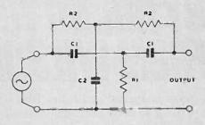
$f = \frac{1}{2}\pi C_1 R_2 \qquad R_2 = 2R_1 C_2 = 2C_1 \\ = \frac{1}{2}\pi C_2 R_1$
