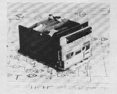
totally self-contained unit requiring only connection to 5 and 12 volts dc. This deck is capable of recording at speeds of up to 25 8 bit characters per second.
