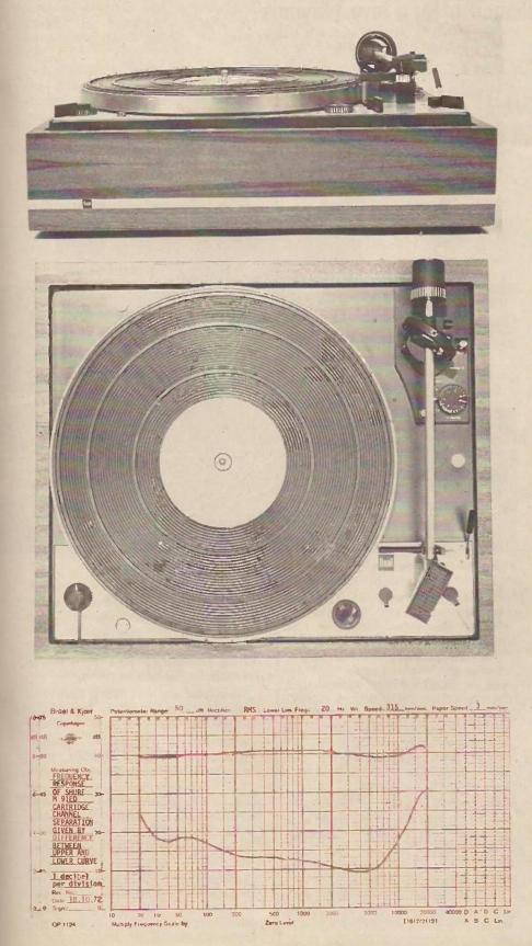
behind the record size select lever. This is very well damped in the raising mode and partially damped in the lowering mode. Two further controls are located at the base of the tone arm pivot and consist of an antiskate adjustment and a lever for raising the gimbal joint to compensate for a multiple stack of records.
