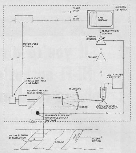
Fig. 6. Schematic of airborne thermal scanning apparatus used in remote sensing for civil and military purposes.
