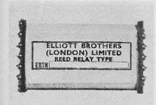
A comprehensive selection of fifteen coils is available with each of the four form styles offered, nominal operating supplies being 5 fo 110 V dc. The dry reed contacts have ac and dc resistive load switching capacities of 80 VA and 30 W respectively, a maximum permissible switching current of 1.5 A, constant current of 2A maximum, a switching voltage of 220 V dc to 60 Hz, and a minimum breakdown voltage of 490 V peak in their activated condition (560 V peak nonactivated).
