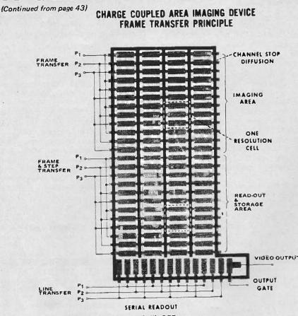
Fig 5 - Frame transfer principle in Bell's CCD sensor
