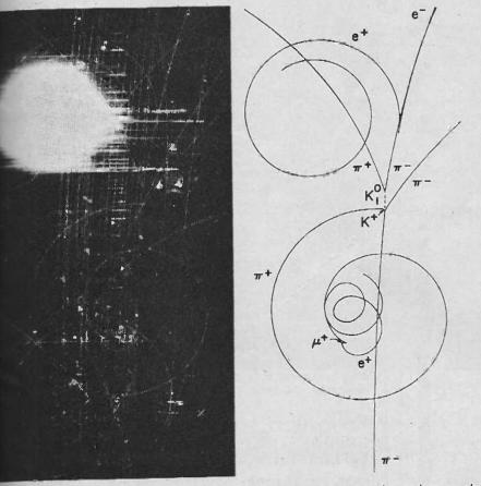
Simultaneous creation of matter and antimatter: gamma ray decays into an electror  $(e^-)$  – positron  $(e^+)$  pair.
