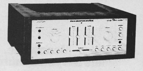
Latest amplifier from Marantz has 120 watts output per channel.
