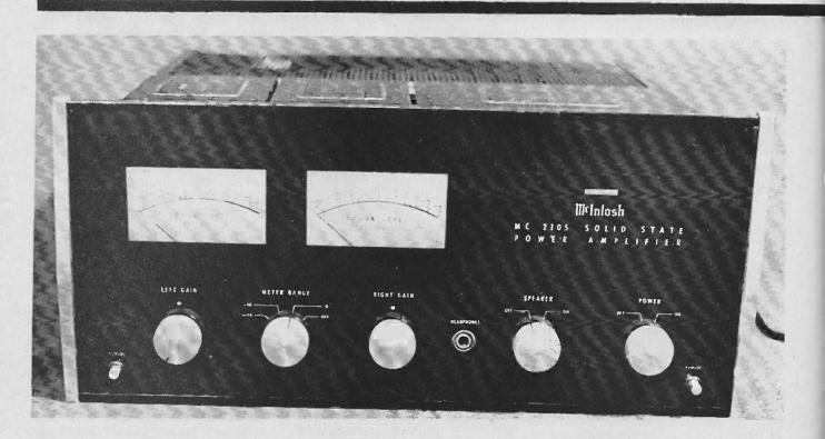
THE McIntosh MC2105 solid state power amplifier is very similar in appearance to the preamplifier. The external finish is identical, with a black glass front panel with chromed trims at each end and machined aluminium knobs.
