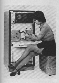
The System 2001 uses a Tally high speed paper tape reader to input data to the Kennedy Magnetic Tape unit at a speed of 500 characters/second.
