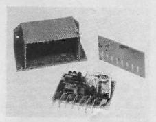
Made of High Impact Polystyrene, it measures 90 x 50 x 37 mm including mounting flanges and has an internal volume of 10 cc. Among various unique features, it has facility for 2 printed circuit boards on which miniature mains transformers and relays may be mounted. Printed circuit fast-on connectors and snap-fit lid eliminate the need for a special plug and socket. Available in 5 different colours
