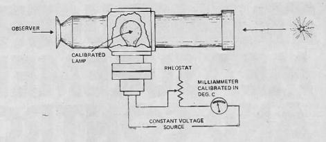
Fig. 2. The basic disappearing-filament optical pyrometer — the rheostat is adjusted until the light filament just disappears. Temperature is read from the dial.
