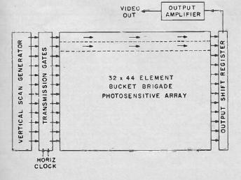
Fig 3 – Block diagram of a BBD charge-transfer sensor
