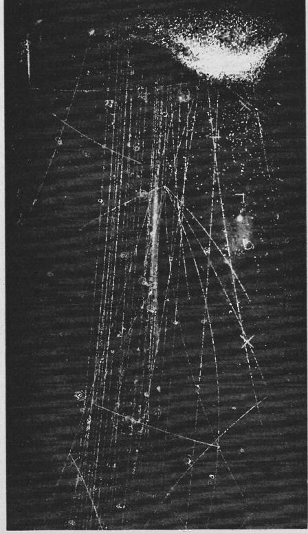
Proton-antiproton annihilation in a liquid hydrogen bubble chamber.
