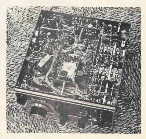
permeability-tuned T notch filter to the first IF amplifier. The IF amplifier has an IF tuner incorporating four high Q, LC circuits which utilise gauged permeability-tuning to obtain four bandwidths of 0.4, 1.2, 2.4 and 4.8 kHz at the 6dB points.
