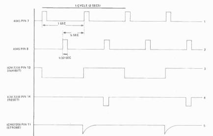
pulse (waveform 3). Waveforms 2 and 3 are NANDed into pin 14 of the ICM 7208s counter chip to produce the RESET signal. Waveform 3 is also inverted before driving a differentiator
