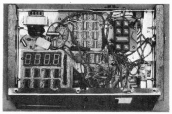
Top view of the completed unit. The crystal oscillator can be seen, bottom right, and the switch bank, top right.
