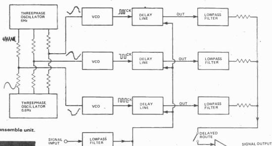
Fig. 5. Block diagram of the ensemble unit.
