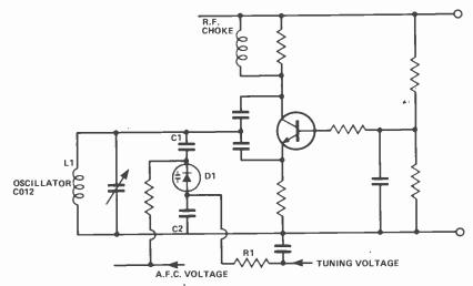
Fig. 9. The varicap diode, D1, is in series with C1 and C2, and is part of the tuning capacitance for L1. Since the diode capaciance is varied by the control voltage from R1, tuning can be carried out by altering this DC voltage.
