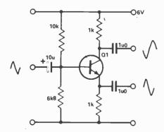
Fig. 9. The transistor phase-splitter.
