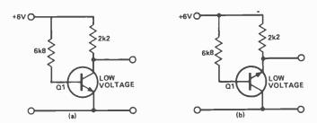
Fig. 7. Obtaining very low stabilised voltages (a) conventional method, (b) using an 'inverted' transistor for lower voltage output.
