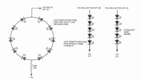
Fig. 3. LED configurations for the bass and treble lines.
