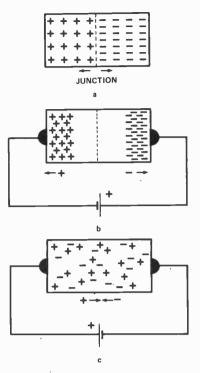
Fig. 4. When a junction is formed (a) the electrons and holes separate slightly at the junction. Reverse bias (b) makes the separation much greater so that the material can't conduct — there aren't any carriers. Forward bias (c) allows electrons and holes to cross the junction, making the material a conductor.
