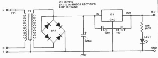
Fig. 5. Circuit diagram of the power supply.
