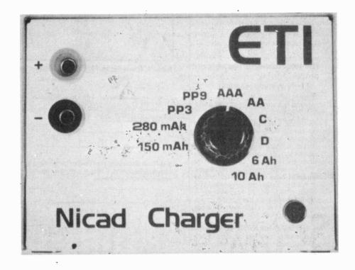
nicad charger is designed with this criteria in mind. It will comfortably charge up to six cells in series (of the same type) at a rate of  $\frac{c}{16}$  amps
