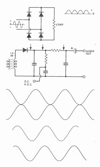
Fig. 5. Using diodes (a) for rectification (b) for radio signal detection. Both applications depend on the one-way flow of current through the diode.
