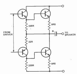
Fig. 15. A quasi-complementary output stage. The power transistors can both be NPN types.
