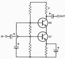
Fig. 16. A cascade stage. The load Z can be a tuned circuit or a high-value resistor providing the bias resistors are chosen to suit.
