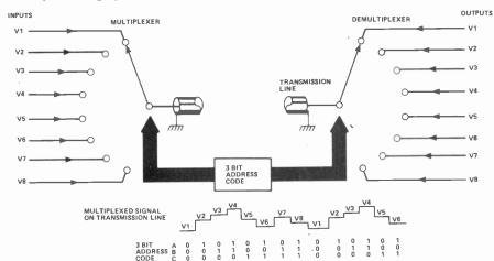
Fig. 2. The principle of the multiplexing / demultiplexing system.
