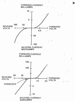
Fig. 3. Forward and reverse characteristics plotted on one graph. (a) Germanium diode, (b) Silicon diode. Notice that the scales for reverse voltage and current are *not* the same as the scales for forward voltage and current. This has to be done so as to get the two different characteristics on the same graph.
