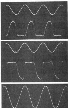
Adjusting bias voltage on the delay lines (chorus board). In each case the top trace is the input signal. The lower trace indicates (a) bias too negative (b) bias too positive (c) correct bias, symmetrical clipping.
