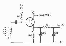
Fig. 2. Using the base/emitter junction of a transistor as a detector diode. The 1M resistor keeps the junction slightly conducting, so increasing the sensitivity.
