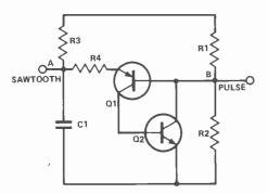
Fig. 12. A two-transistor equivalent of a unijunction.
