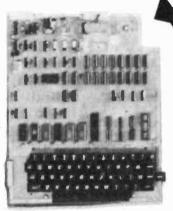
This 6502 based microcomputer comes with a full 8K Microsoft basic in ROM. Full keyboard. 4K static user RAM (on board expandable to 8K). Kansas City standard interface for use with an ordinary cassette recorder. Machine code monitor and I/O utilities in ROM. Direct Video access with 1K dedicated RAM (besides 4K user RAM) and full graphics set.
