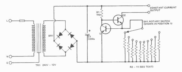
Fig 3. Circuit diagram for the ETI Charger. Resistor values are given in the text for the charger resistors.
