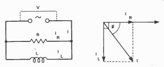
Fig. 5. (a) A resistor and an inductor in parallel. In this case voltage is used as the reference quantity. (b) The phase diagram for a parallel L-R circuit.
