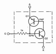
Fig. 13. Using two transistors in place of a thyristor.
