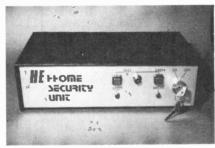
Well, we couldn't call this project a mere burglar alarm. It boasts a 'panic button', fire alarm option and as a further bonus it will drive either a mechanical bell or the electronic siren we're incorporating into the design.
