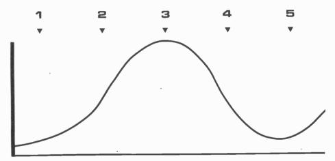
Fig. 1. Bass and treble signals are shown in the graphs, top and above respectively. At point 1, with a lot of bass and very little treble, pattern 1 of LEDs light (shown left), and so on. Thus the pattern of LEDs changes, with the changing mixture of bass and treble frequencies.
