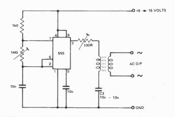
Many home-grown projects require a high voltage, low current source. The simplest and safest means of providing this is by an inverter. The circuit described here is versatile, efficient and easily capable of providing power for portable Geiger counters, dosimeter chargers, high resistance meters, etc.
