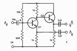
Fig. 10. Modified phase-splitter with equal output resistances.
