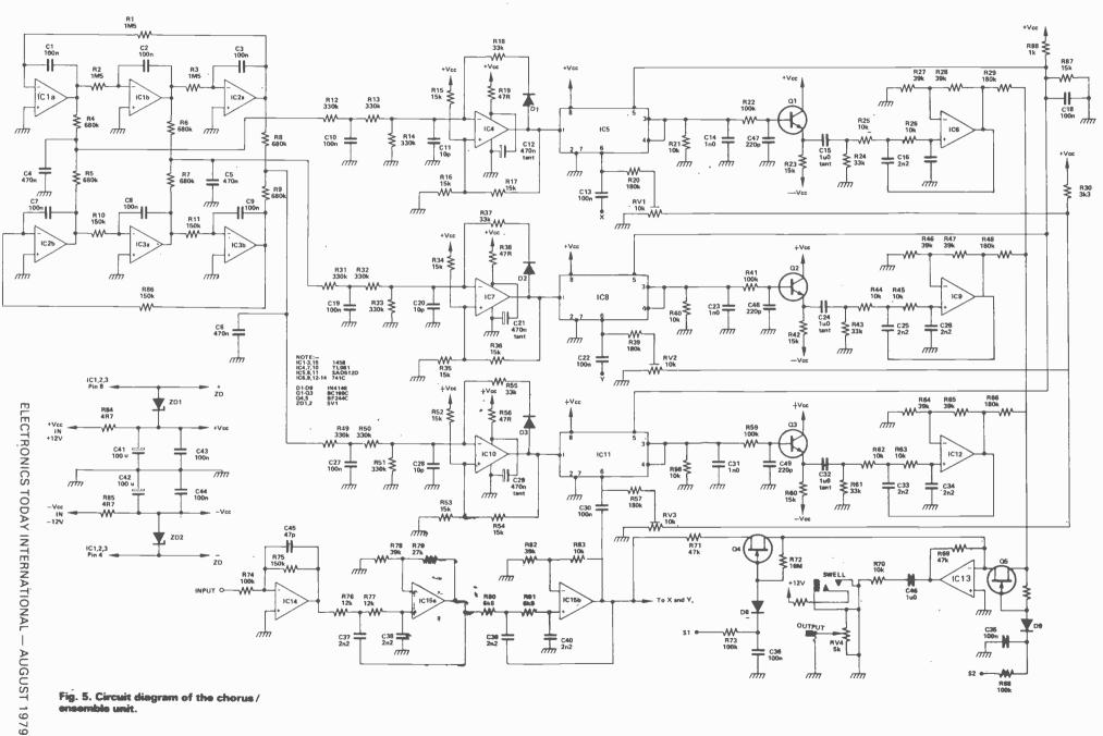
Fig. 5. Circuit diagram of the chorus/ ensemble unit.
