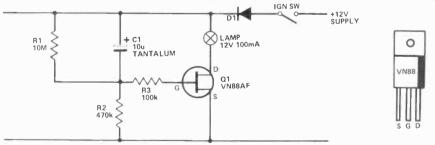
across a capacitor cannot change instantaneously (C1 is discharged by R1 when the supply is removed). As the capacitor charges up the gate potential of Q1 drops and the lamp extinguishes. The current drawn by
