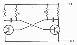
Fig. 6. Conventional multivibrator circuit.
