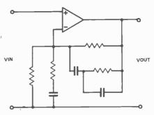
Fig. 4. An operational amplifier with equalization circuitry in its feedback
