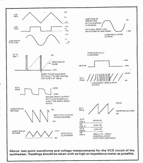
(RV14), and the sine wave voltage from the slow oscillator. The output from this circuit is limited to a range of 0 V to about —10 V. As the manual shape pot is rotated clockwise the waveform at the junction of R57, R59 will change from a ramp into a triangle, this being due to the full wave rectification. With RV14 fully clockwise and RV15 anticlockwise adjust RV15 so that the waveform is a symmetrical triangle.
