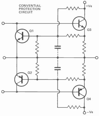
A study of the circuit of a conventional V-I protection circuit will show that as the protection transistors turn-on they become a 'non-linear resistor' across the bases of output transistors Q3 and Q4 and as such create unpleasant distortion. One solution tried by some companies was to slug the bases of Q1 and Q2 with a capacitor to provide a time-delay to prevent the protection operating except during a sustained short-circuit.
