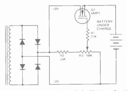
Fig. 16. Tapered-current voltage-limited battery charger.
