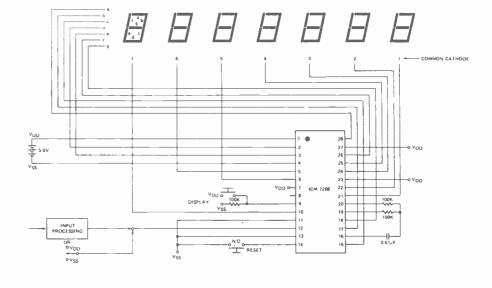
Fig. 5. Unit counter schematic.
