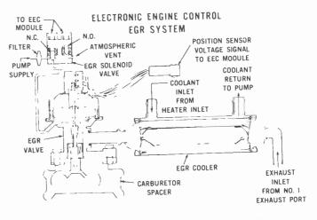
Fig. 6. Above, diagram of the Electronic Engine control system featured in the 1978 Lincoln Versaille.
