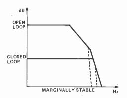
In the case of the inconditionally stable amplifier the only ill-effect will be some "ringing" in the closed loop step response — but in the case of the marginally stable amplifier it may go completely unstable. The most popular "belt and braces" solution to this problem is to fit a resistor-inductor network at the output to "cancelout" the effect of the capacitive loading, thus
