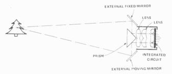
Fig. 1. External arrangement of mirrors for the Visitronic
