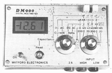
Fig. 1. View of the final unit. Note, in order to ensure that the input sockets do not foul the PCB yet allow the probes to be inserted, the sockets should be mounted 10mm from the bottom of the case.
