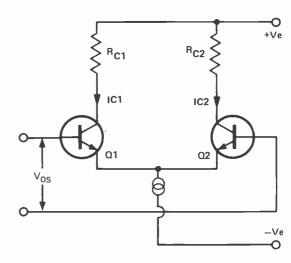
In this circuit the input offset voltage is related to the base-emitter voltage of this transistor.
