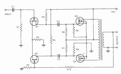
Fig. 12. Transformer-coupled output.
