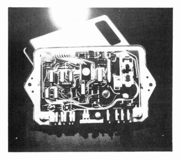
Fig. 1. Left, a Delco Remy module, part of an electronic controller for the GN 3-way catalyst system.
