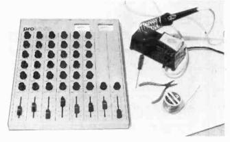
R E W Audio Visual have been given exclusive distribution rights on a new kit for budding rock & roll stars in the U.K Called Prokit 62, it is a 6 into 2 audio mixer with features not normally found on mixers in the sub £100 range (at £99.95 it just creeps into this bracket). Each input channel has bass and treble equalisation, pan control, echo and cue busses, with choice of line or mike inputs. Distortion is claimed to be less
