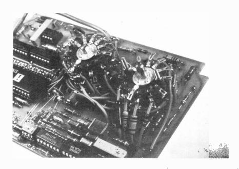
is obtained. If 1% resistors have been used where specified, changing to the next range should give a reading of exactly one tenth, and the next one hundredth, allowing for the plus or minus one digit accuracy. Calibration should ideally be done on the 200 mV range since this does not involve the attenuator, but this is not
