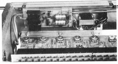
Above: close up of the PSU board mounting within the case. Positioning the transformer is important to reduce the risk of hum. Mount this as low down, away from the board, as possible. In the foreground the resistor chain for the keyboard can be seen. Below: overall
