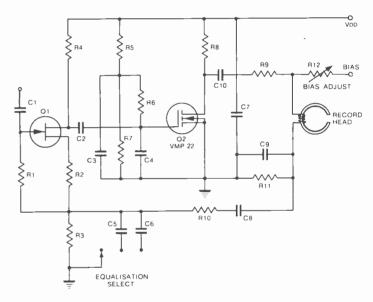
Fig. 13. Tape recording amplifier.
