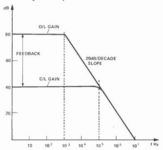
In the case shown in the diagram (unconditional stability) the open-ioop response of the amplifier is stabilised by rolling it off at a slow 20 dB/decade slope with a single pole at 1 KHz. This amplifier would be stable with any amount of resistive feedback. However it will be seen that at higher audio frequencies the amount of feedback available reduces and so the distortion of the amplifier will increase. For this reason many amplifiers are of the "marginally stable" type.
