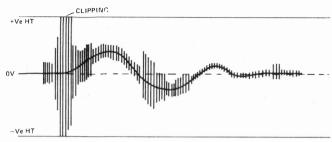
Effect of a sine wave of varying amplitude as signal upon the DC offset voltage at the output.
