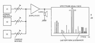
Intermodulation distortion testing using three frequencies.
