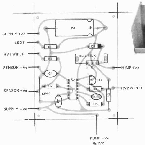
Below is the complete system, the probe used was made from a jack plug. On the right is the PCB shown full size (70mm by 90mm).
