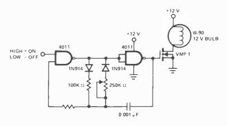
Fig. 8. Circuit of a high-efficiency light dimmer.
