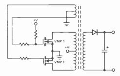
Fig. 10. A DC to DC converter (Siliconix).
