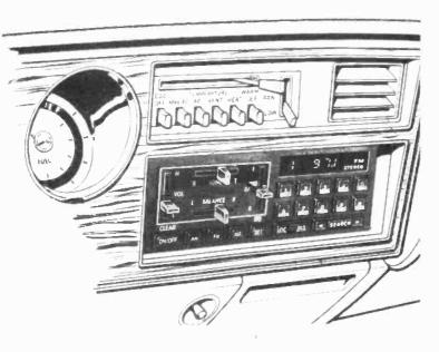
internal memory. A LED display shows the frequency and number of the selected station.
