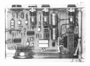
To the left we see the ultra sonic receiver from above. We glued the ultrasonic transducer in place but it would be preferable to insulate this from the rest of the case with foam rubber. The picture on the right shows the transmitter out of its shell.
