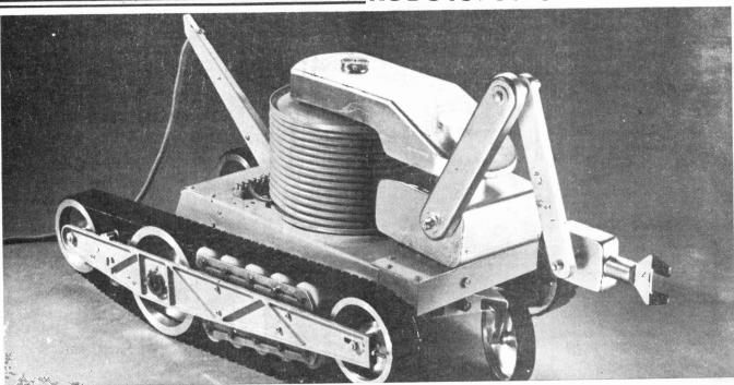
Fig. 2. (left). HORACE, a Warwick University Robot Laboratory mobile, is simple to make and uses commercial parts. Robots like this are well within the scope of amateurs. Note the ease of access to parts.
