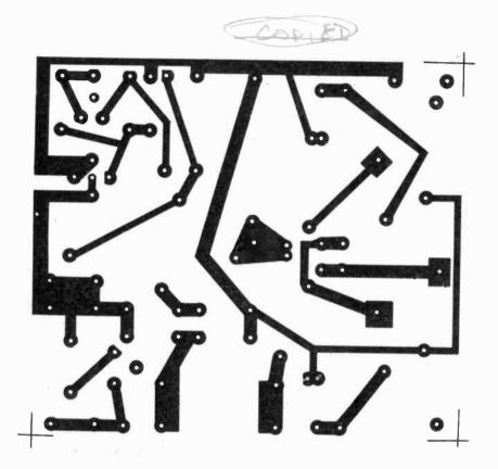
Fig 1. Foil pattern for the ignition's PCB.
