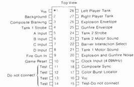
Fig 3. 8710 pinout.
