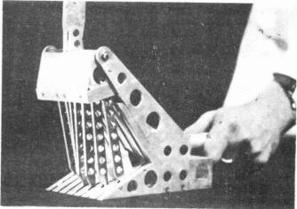
Fig. 2. Prototype mechanical hand for use with robots.
