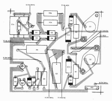
Fig. 2. Component overlay of the CDI.
