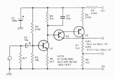
emitter mode. Heavy local AC and DC feedback is introduced by R5 and this defines the gain of the stage at 20dB. To minimise noise a BC109C is used here operated with a low collector current, 50uA. The output stage of this amplifier is the darlington pair Q2
