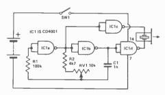
Fig. 5. The circuit of the ultrasonic transmitter
