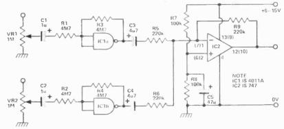
power supply is used the noninverting input must be biased at half the supply voltage. This is done by the couples this point to earth.
