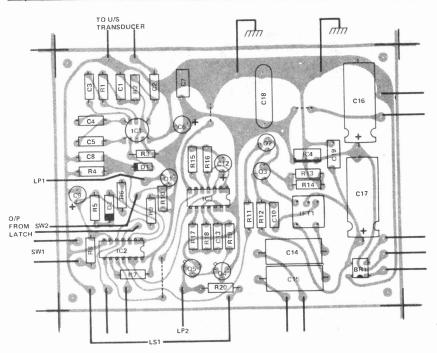
Fig. 1. Overlay of the ultrasonic receiver board.
