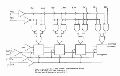
Fig 4. Schematic diagram of the 7494 shift register. Compare the number of flip-flops gates and inverters in this single chip with the number pf packages needed to make this from 7400's and 7476's.
