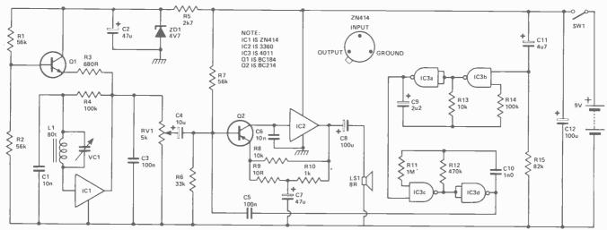
Fig. 1. Circuit diagram of the Star Trek radio.
