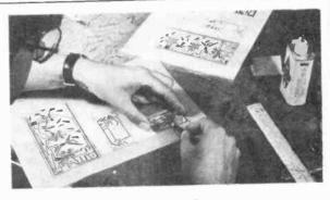
Lay down the ETIPRINT and rub over with a soft pencil until the pattern is transferred to the board. Peel off the backing sheet carefully making sure that the resist has transferred. If you've been a bit careless there's even a 'repair kit' on the sheet to correct any breaks!
