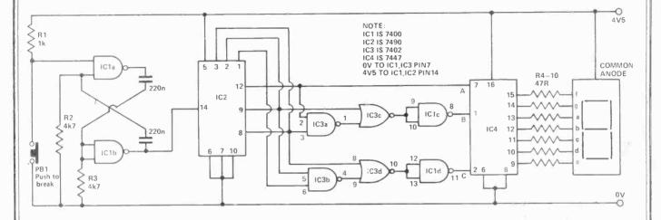
ICla and IClb form an oscillator running at a few kilohertz. The output is fed to a 7490 binary counter which is wired to produce an output of 0 to 5 in BCD. So that the display is the same
