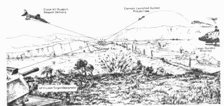
More from 'Star Wars' Ferranti — this time a laser system for tanks. The applications of the laser transceiver include automatic ranging and laser target designation (in which a beam fired from the tank is scattered from the target and picked up by a guided missile). The specifications of the system are:
