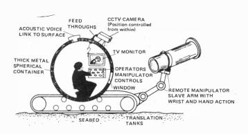
Fig. 3. Underwater a robot manipulator provides an operator with an effective ecoskin and increased ability to do work.
