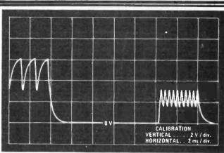
Fig. 2a Waveform on pins 2 and 6 of IC3.
