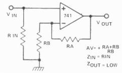
Fig. 8. Non-inverting amplifier.
