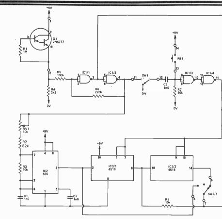
Fig. 1. Circuit diagram of the timer.
