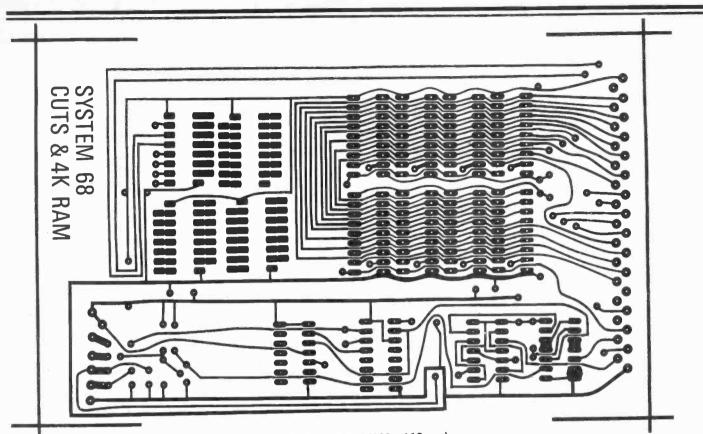
Fig. 1. Foil pattern for CUTS and RAM card shown full size (160 x 110 mm)
