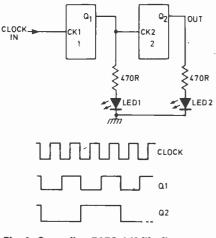
Fig. 1. Cascading 7476 J-K flip-flops. (a) Circuit. (b) Pulse diagram.
