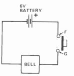
DC supply is used take care to ensure that the positive side of the push is connected to point F
