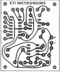
Fig. 4. Printed circuit layout. Full size 60 x 50 mm.
