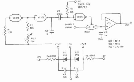
voltage input is therefore sampled and the value of the amplitude at this point of the waveform is remembered by the high input impedance ( $10^{12}$  Ohms) CA3140 voltage follower. This output is then used to control the VCO etc. The oscillator and monostable can be constructed from either a CMOS 4001 or 4069, ensuring that unused pins are connected to the high or low power supply line via a 1k resistor. The input waveform to the analogue switch can have an amplitude of  $\pm$  7 V maximum.
