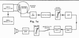
Fig 1. a) On the left shows the block diagram of the Mark 1. In this the peaks of the modulated signal were gated and enormously amplified. On the right is shown the new arrangement, the RF signal, which is unmodulated, is converted to a DC signal which drives a voltage controlled oscillator (VCO).
