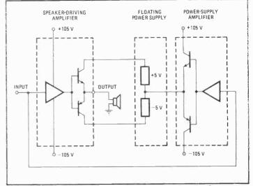
Block diagram of the Matsushita 350W amplifier circuit which is designated A+.
