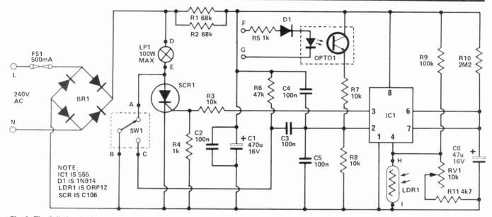
Fig. 1. The full circuit diagram of the Porch Light is shown above.
