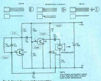
Fig. 2. Circuit diagram of the transmitter.
