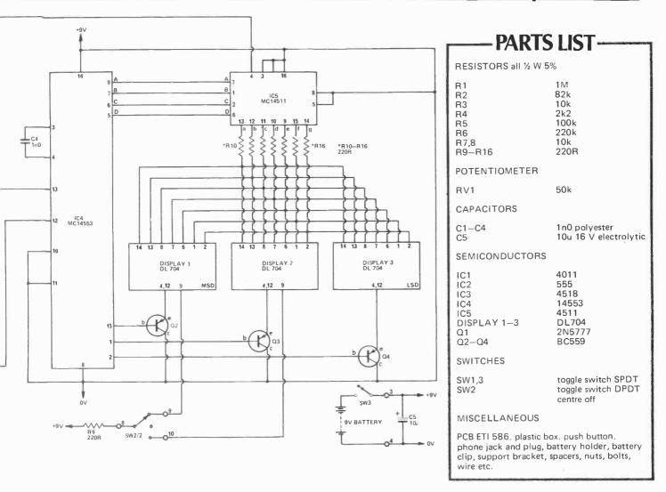
Fig. 2. Component overlay and wiring diagram.
