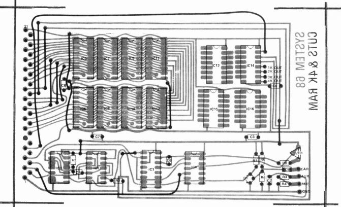
Fig. 2. Overlay for CUTS and RAM card.
