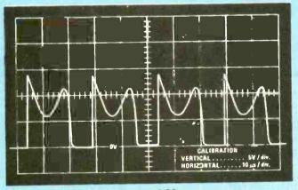
Fig. 3c. Voltage on the collector of Q2.
