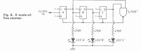
Now apply power and check that the count sequence is as shown in the truth table of Fig. 3 when the gating switch is ON. Try switching the gate off and resetting.
