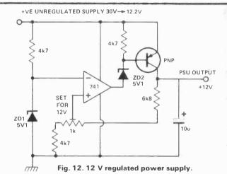
allows the op-amp output to work at about 7 volts below the unregulated supply rail. Thus, a regulated output is maintained until the PNP transistor saturates. This means that the unregulated rail can fall to within about 200 mV of the regulated rail!
