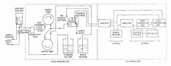
Fig. 6. Schematic flow diagram of console used to operate a chosen selective-ion probe under automatic conditions (EIL).
