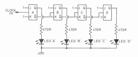
Fig. 4. Cascading from the  $\overline{\mathbf{Q}}$  terminals — what does this counter do?
