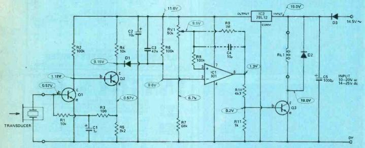
Fig. 1. Circuit diagram of the receiver.
