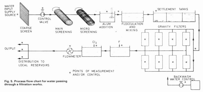
temperature, conductivity, suspended solids, and ammonia and nitrate levels dissolved in the water. Flow rate is also gauged.
