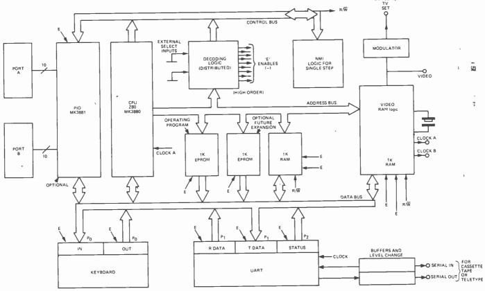
Fig. 1. A block diagram of the NASCOM 1 system. ELECTRONICS TODAY INTERNATIONAL - FEBRUARY 1978
