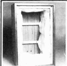
Fig 2. Internal shot with the wadding fitted to the sides. The back panel has not yet been lined. The bracing across the panel can be seen, and this continues around the sides.
