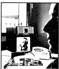
Fig. 2. Video links provide a greater communication capability but require more bandwidth than a telephone. (This Siemens experimental system uses 1 MHz).
