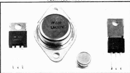
This three terminal, positive voltage regulator, capable of supplying in excess of 1.5 amps, and adjustable over an output range of 1.2V to 37V, has recently been announced by Jermyn. Requiring only two external resistors to set the output voltage, the LM317 has typical line and load regulation figures of 0.01%V and 0.1V acteristics to those of most standard
