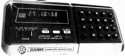
You can set 4 separate alarms and the time is accurate to ±15 seconds per month (0° - 40°C). The 199 year calender compensates for varying month lengths and leap years.
