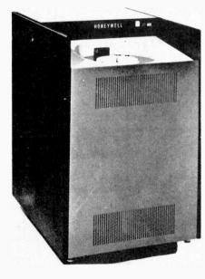
Fig.2. Honeywell model 4720 movinghead disk storage device.
