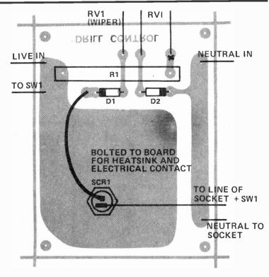
Component overlay for Speed Controller Parts List-
