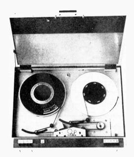
Fig. 1. The Hewlett-Packard 7970 magnetic tape unit designed as a peripheral to EDP systems.
