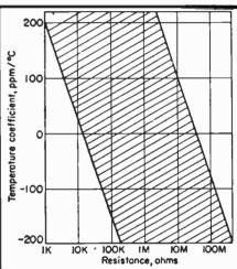
Fig. 1. Range of temperature coefficients available for various values of metal film resistors having controlled TC characteristics
