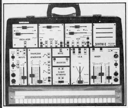
EMS have produced a small-scale synthesizer especially for school usage. ical keyboard (3 octave). oscilloscope, It arrives with a comprehensive teaching course, and is of modular construction, such that patchcords are required EMS Ltd., 277 Putney Bridge Road, for linkage.
