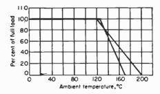
Fig. 4 Two typical derating curves from different manufacturers for Mil-spec metal film resistors.
