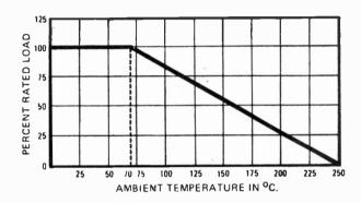
Fig. 7. Derating curve for square-section style power metal oxide film resistors
