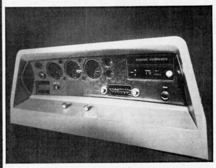
This mock-up has been put together by Bowmar Instruments to show one very possible future of the car dashboard. It includes both circular and linear bargraphs along with digital and alpha-numeric displays. All the
