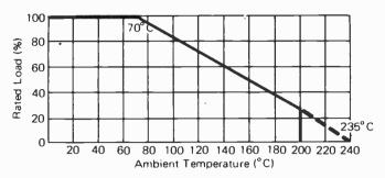
Fig. 6 Derating curve for cylindrical style metal oxide film resistors with ratings between 1 W and 7 W.
