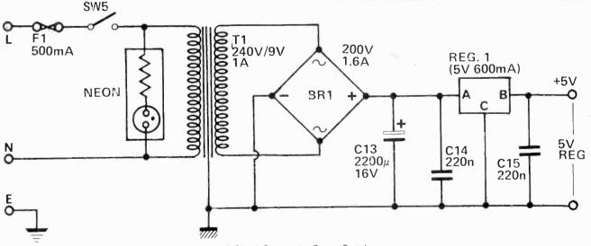
Fig 9 Circuit Diagram - Power Supply
