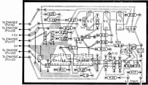
Fig 4: Overlay —Analogue Board
