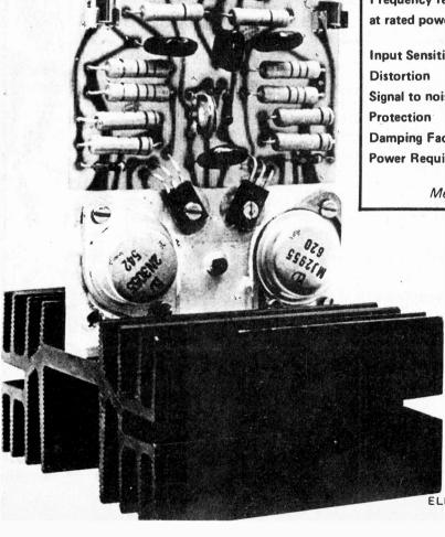
The screws holding the 2N3055/MJ 2955 should also be insulated where they pass through the heatsink bracket. The BD 139 and BD 140 do not need any insulation other than the mica, provided 6 BA (or 3mm) screws are used. In the 100W version the additional transistors are mounted on the heatsink bracket outside the PC board area.
