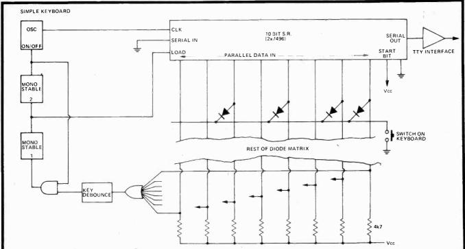
Figure 2: A simple keyboard. The circuit shows how pressing one key sets up a parallel code and instigates operation of the serial code generator. This circuit outputs an eleven-bit serial code: first a start bit (logical zero), then eight bits taken from the ASCII code, then two stop bits (logical one). To do this the shift register needs 11 clock cycles but if it gets more it doesn't matter with this circuit, it just gives out more ones. See figure 3.
