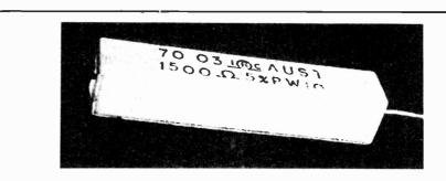
Fig. 5. Square section, 'ceramic boat' style medium power film resistor
