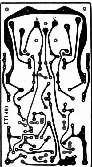
Printed circuit layout of the amplifier. Full size 140mm x 76mm.
