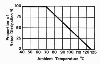
Fig. 3. Derating curve for some types of miniature 1/10 W, 1/8 W and 1/4 W metal film resistors.
