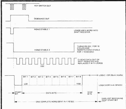
Figure 3: These waveforms show how the circuit in figure 2 works. The final waveform is that expected by the interface and monitor programs of the evaluation kits — it is the format used by a teleprinter to send and receive in ASCII.
