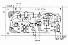
PCB Overlay For The Function Generator
