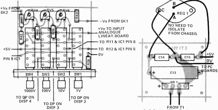
Fig 7: Overlay - Input Switching Board
