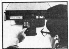
Both of the first models in the range to be announced (9015 and 9035) work to 100MHz in measuring frequency, period, period average, time interval, time interval average, frequency ratio and total count. Thanks to the microprocesor direct readout of preset operations, reciprocal calculations, and even answers in engineering units are easily achieved. 9-digit constants can operate on measurements through the keyboard.
