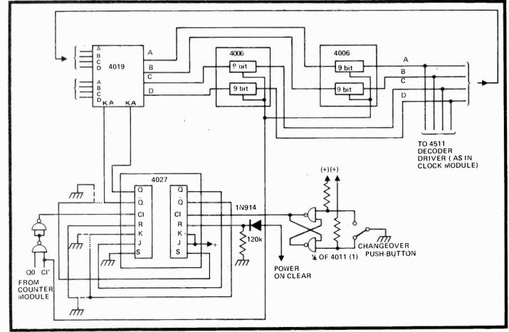
Fig. 8. Circuit diagram of the latch.
