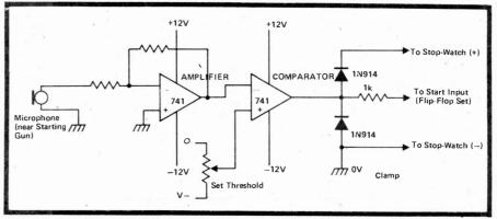
Fig. 10. A simple circuit for using the sound of a starting gun to start the Stopwatch.
