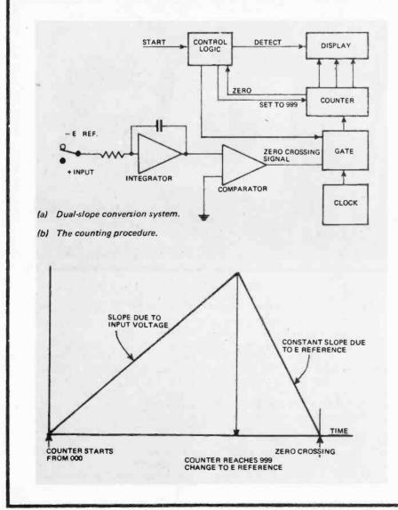
Initially when an unknown voltage is applied to the input a 'start conversion' pulse is generated and simultaneously all the counters are set to zero.
