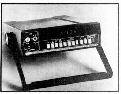
The Fluke 8000A digital multimeter offers 0.1% accuracy with three and a half digits.
