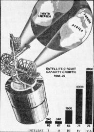
2.35 meters. Solar panels, covered with 17,000 solar cells, provide the craft with primary power of 600 watts. The satellite is designed to have an in-orbit life of seven years.
