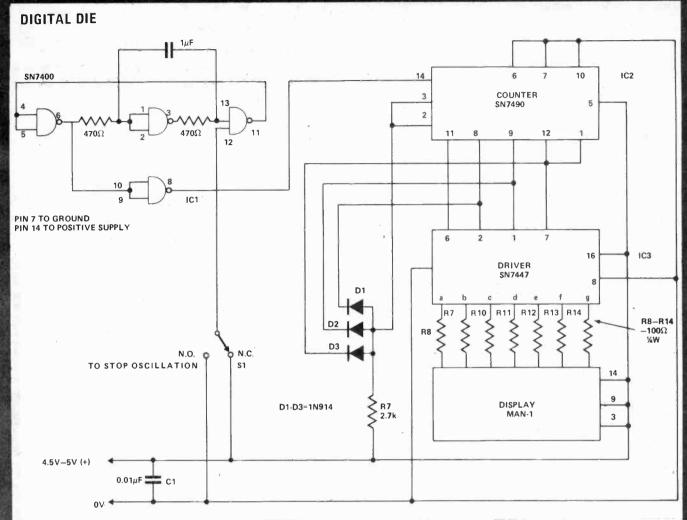
This device is based on a multivibrator (ICI) which has a frequency of about 1kHz. Oscillation continues as long as the input to pin 12 is high; as soon as the input is taken low or connected to earth it stops the cycle. This is used as a stop switch which causes the LED to indicate the random digit.
