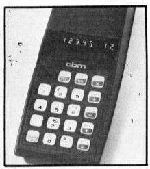
The 8-digit display converts to a 5-digit mantissa plus 2-digit exponent display. It is battery operated with a mains adaptor as an optional extra at  $\pounds 2.50 + VAT$ . The calculator is guaranteed for I year.
