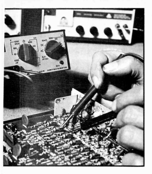
parallel with R2 will produce a combined value of 500 ohms. Thus the voltage read by the meter will be 0.5 volts instead of 0.75 volts – an error of 33 per cent!
