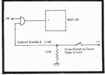
Fig. 12.Controlling the counting with a toggle switch.
