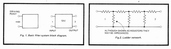
AS WE saw in the previous section resistor-capacitor filters can only provide roll-offs of 6 dB/octave (20 dB/decade. On the other hand combinations of inductors and capacitors can provide much steeper rolls-offs and a response at the turn-over point which can be tailored to a desired shape.
