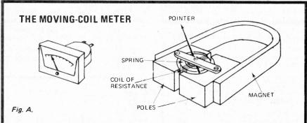
If an electromagnetic coil is suspended in the field of a permanent magnet, it will be caused to rotate, when energized, by a force proportional to the energizing, current.
