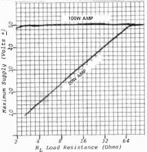
Graph 1: Maximum Allowable Supply (V±) versus load for Sinusoidal Output.
