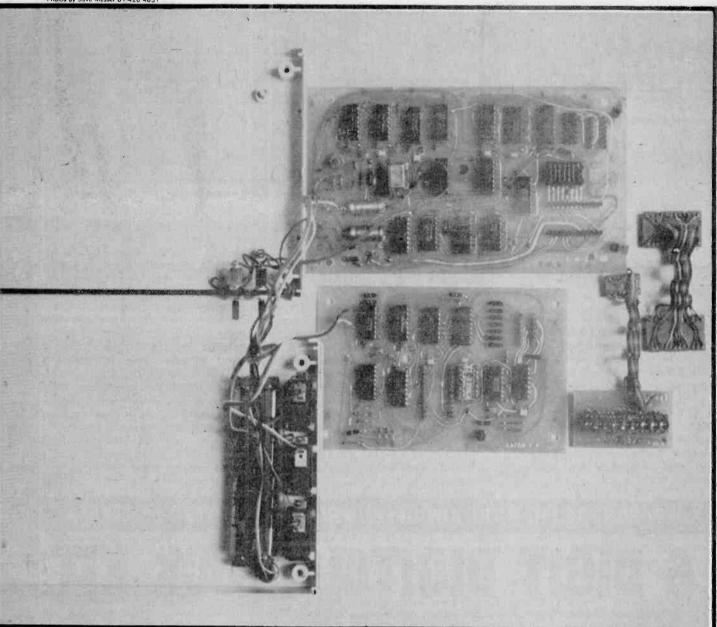
The insides of the stopwatch. The clock board is at the top,the latch beneath. Here we show one display, but a second display module will plug in directly. A small saving can be made by soldering the flat cable directly onto the boards rather than using the LSI plugs as shown.
