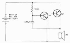
component values shown, a fresh battery or cell will give a note of about 500Hz, whereas an exhausted cell will give a note above 1kHz. The device has been tested with battery voltages between 1.5V and 14V, using a 2N2923 as Q1, and an OC81D as Q2. The unit is undamaged by reversed supply potentials.
