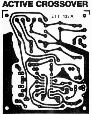
Fig. 5. Printed-circuit layout for the two-way board. Full size 77  $\times$  90 mm.
