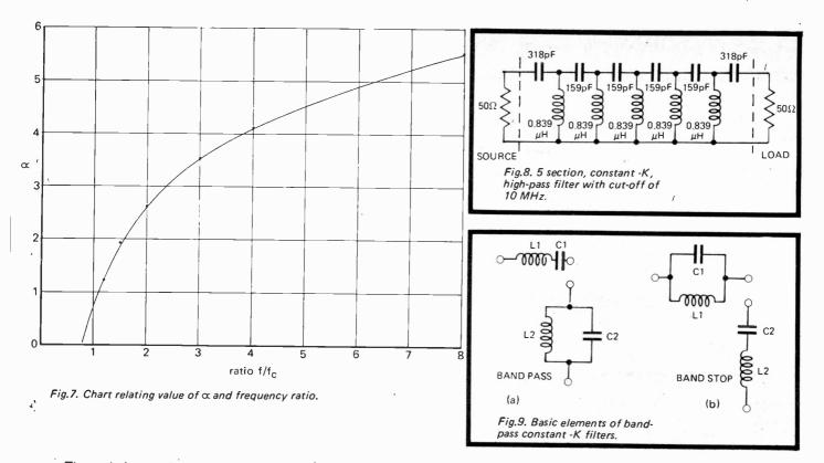
The design of band-pass and band-stop stages is more complicated going beyond the scope of this course. Suffice to say that the components in the arms now become series or parallel resonant combinations. The basic L-section for a constant-K band-pass is shown in Fig. 9a and the basic L-section for a band-stop in Fig. 9b. Readers who wish to pursue these can obtain guidance from the reading list.
