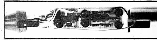
Internal construction of the pulser.
