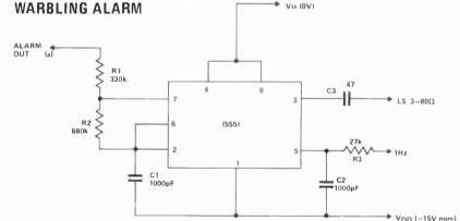
This device gives a two-tone alarm from a digital clock. It may be used with any CMOS alarm clock chip having an active high alarm output and 1Hz (optional) output. It was built to work with a CT7001 chip and requires no interface components.
