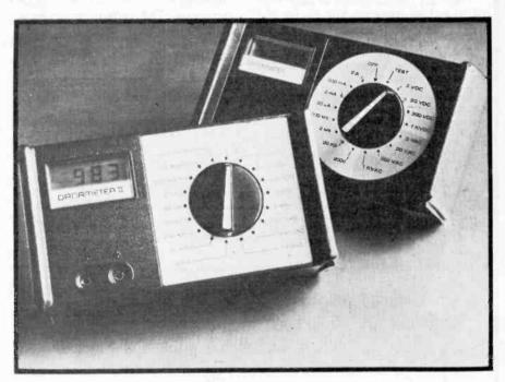
These Danameters are the cheap end of the range from Dana Laboratories. AC accuracy is 1.15% (Danameter) and 0.6% (Danameter II); prices are £135 and £168.50.
