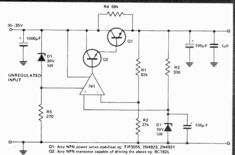
by replacing R1-R2 with a potentiometer, but in its present form, the circuit cannot be made to regulate below the zener voltage of D2. If continuous variation is required, the reference source R3-D2 must be
