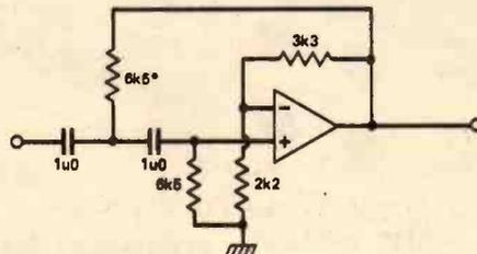
Fig. 4 Circuit for a second-order filter.
