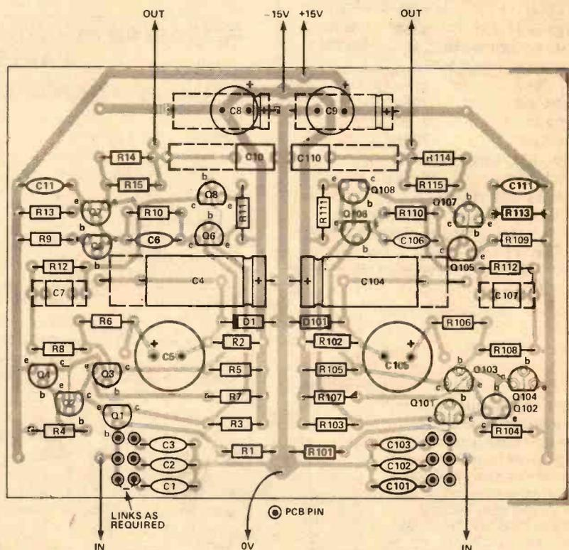
Fig. 3 Full circuit of the PU input stage; note that if you're cutting costs by using 5% resistors, components marked with \*\* must be 2% or better.
