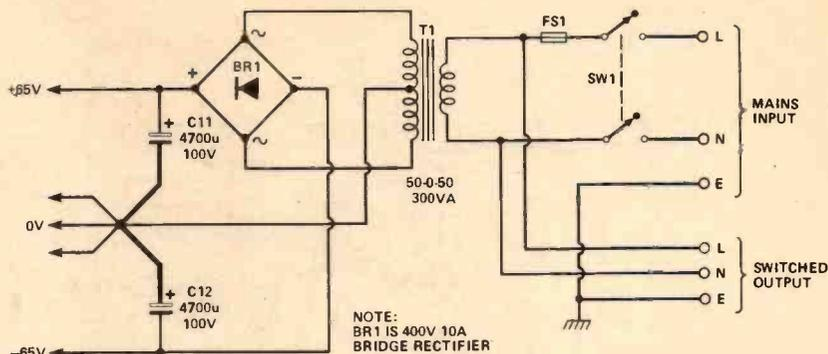
Fig. 7 Mains input circuit for power supplies.
