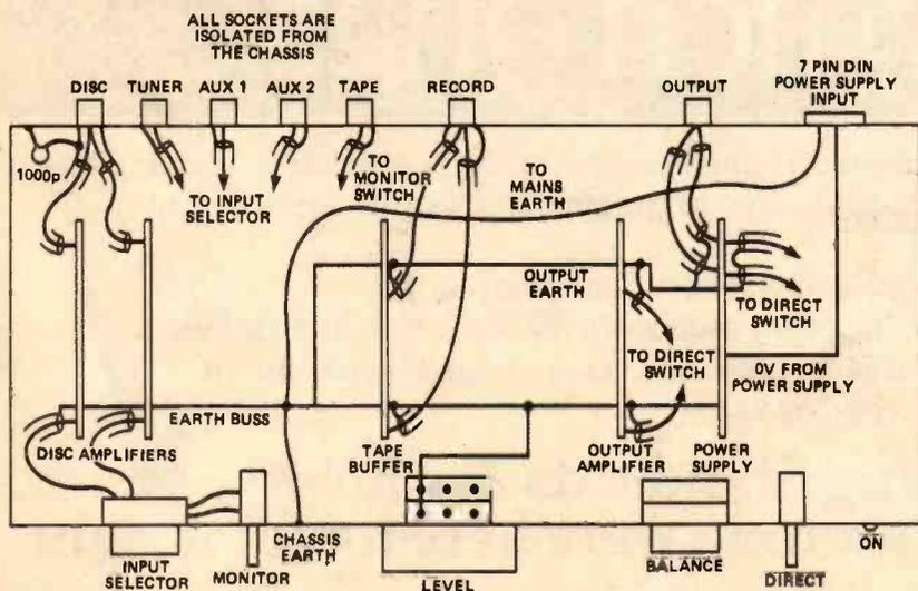
Fig. 11 A possible earthing arrangement.
