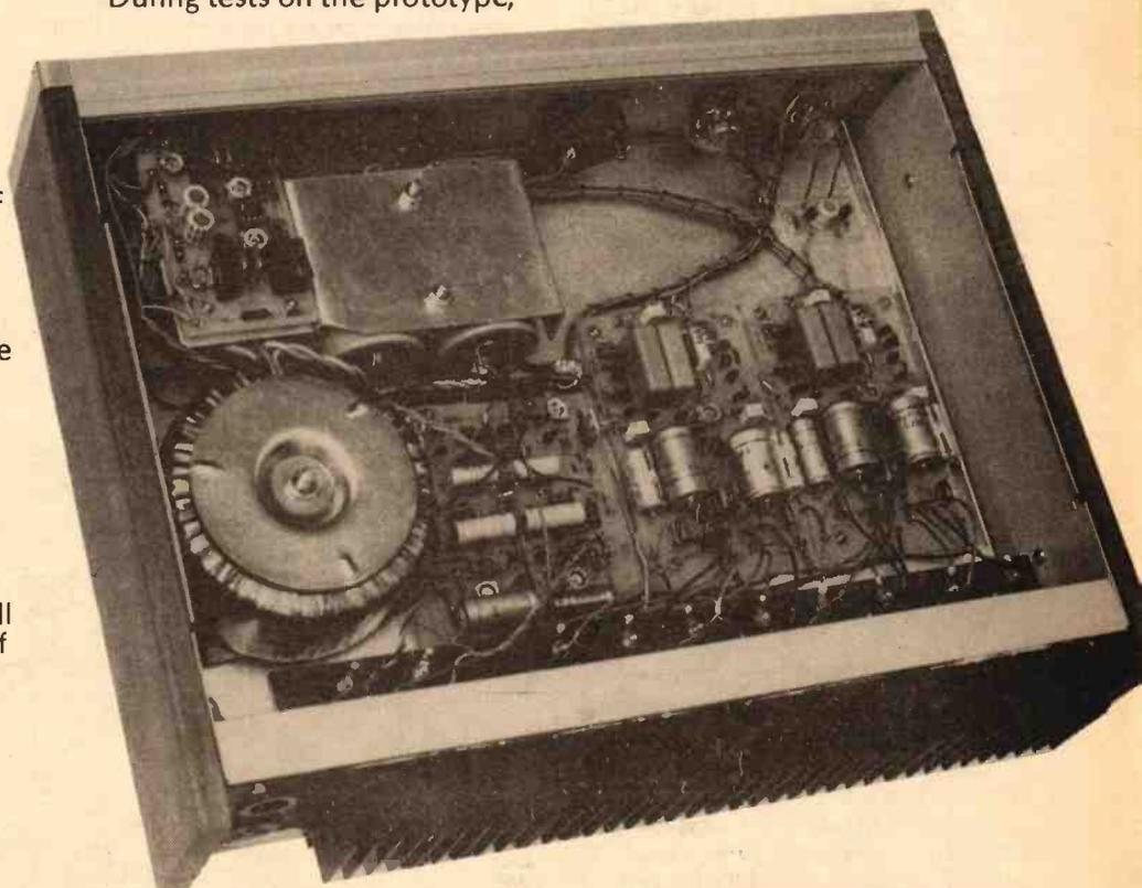
The interior of the prototype: along the top (L to R): meter driver PCB (mounted over on/off and mute switch), reservoir caps, switch-on muting PCB; bottom: transformer, PSU, 2 x power amps
