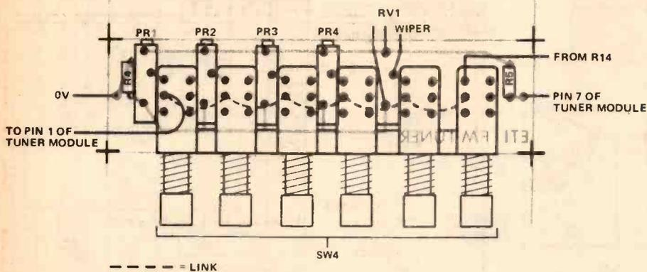
Fig.6 (above) Component overlay of the SW4 six-way switch assembly.
