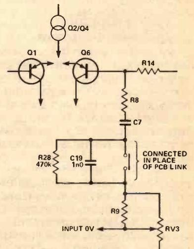
Fig. 10 Circuit arrangement for amplifier muting.
