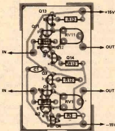
Fig. 4 The overlay diagram of the discrete component buffer.
