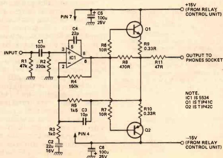
Fig. 8 Circuit diagram of the headphone amplifier module.
