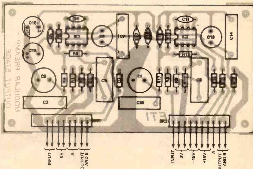
Fig. 5 Component overlay of the unbalanced output stage PCB. Note that this board is for stereo operation and therefore carries two complete output stages.
