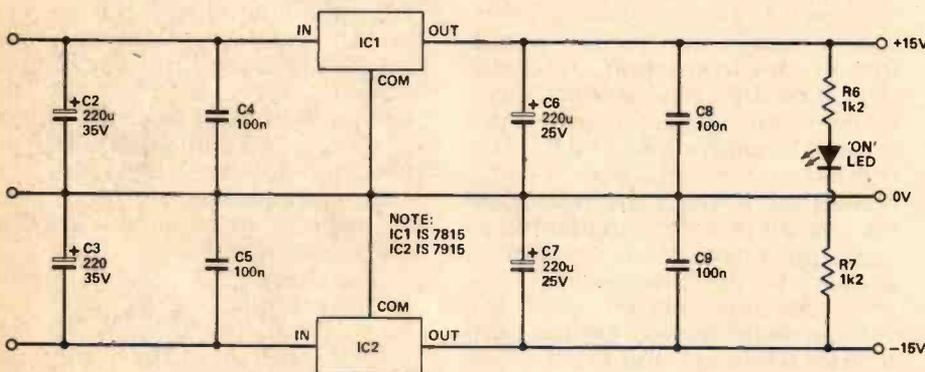
Fig 8. Circuit diagram of the power supply.
