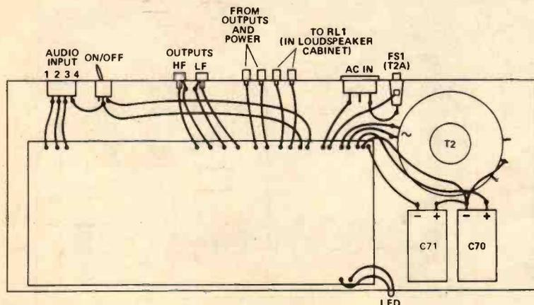
Fig. 4 Internal wiring diagram (note — BR2 not shown).
