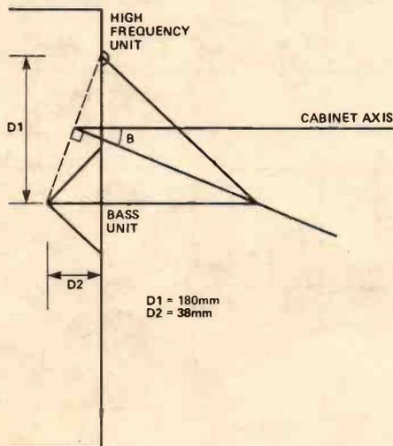
Fig. 10 The effect of the displacement of the speaker coils.
