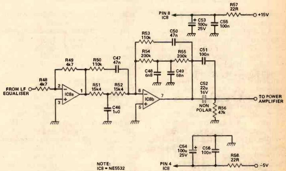
Fig. 12 Low-frequency equaliser for closed-box operation.
