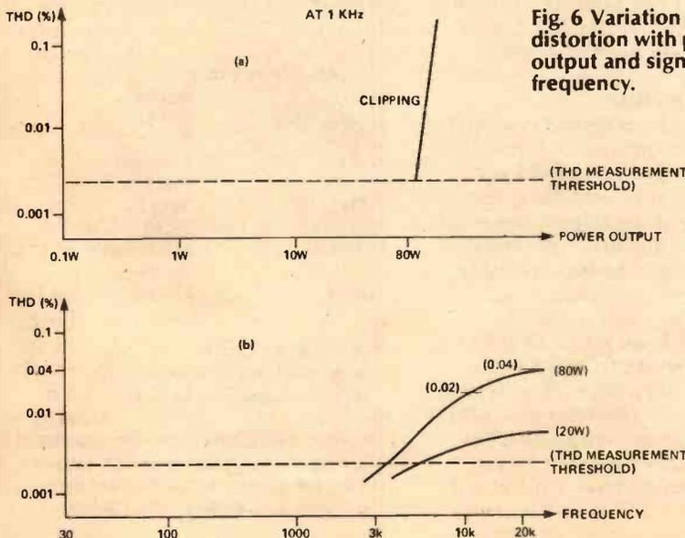
**Fig. 6 Variation of harmonic distortion with power output and signal frequency.**
