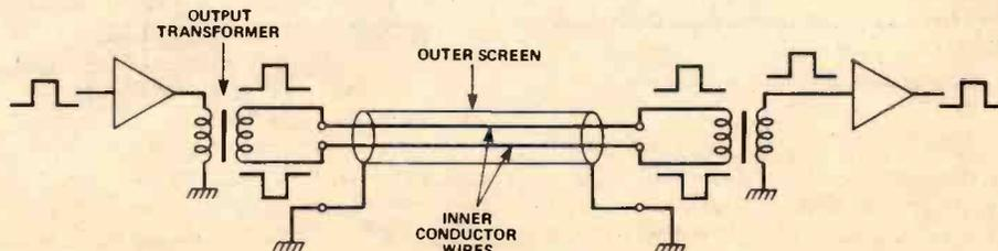
Fig. 4 The basic principle of balanced line operation.
