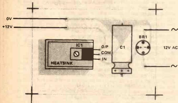
Fig.8 (above) Component overlay of the PSU.
