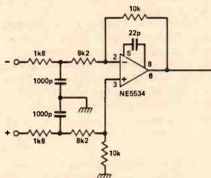
Fig. 7 A possible balanced input arrangement.
