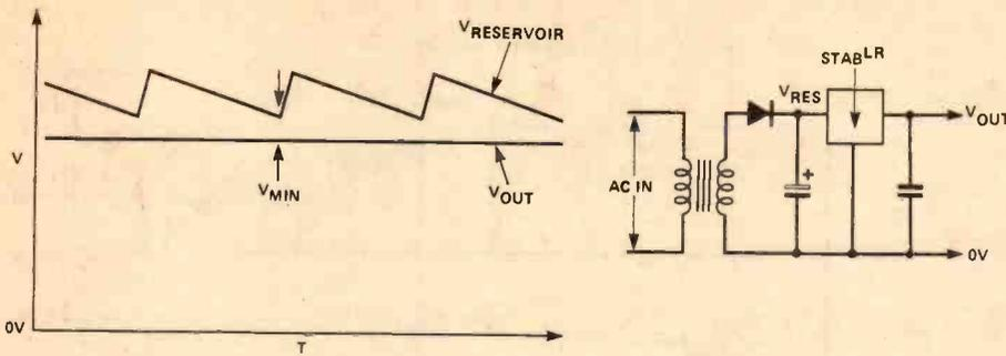
Fig. 2 The effect of ripple on stabiliser input — output voltage.
