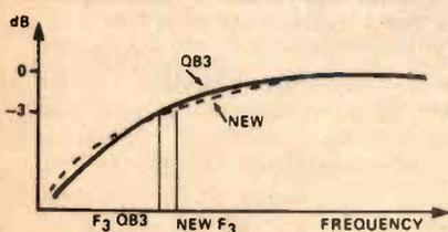
Fig. 4 The response of the V3 speaker compared to the Thiele QB3, showing the improvement in the bass.
