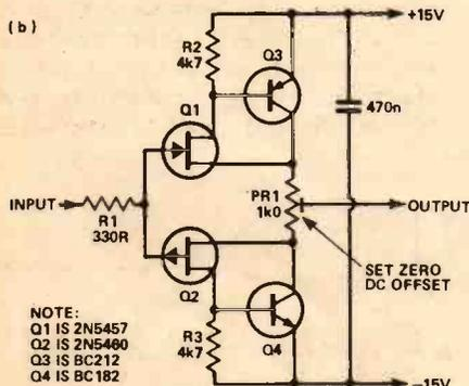
Fig. 2 RIAA stage output buffer options (one channel only shown): (a) using an op-amp,  $Z_{in}$  in excess of 1000 Megohms; (b) using discrete components,  $Z_{in}$  in excess of 100 Megohms.
