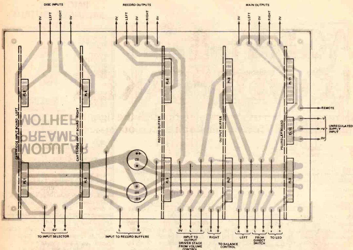
Fig. 4 Here is the overlay diagram for the mother board of the preamp as featured in the first part of the description. We have not reproduced a lay-out for the mother board of the extended system because the whole idea is for it to be adaptable to your needs — so everyone can make up their own, customised preamp using the same basic blocks.
