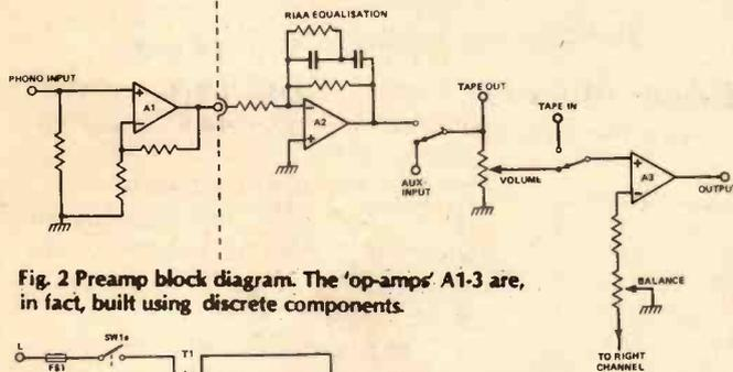
Fig. 2 Preamp block diagram. The 'op-amps' A1-3 are, in fact, built using discrete components.
