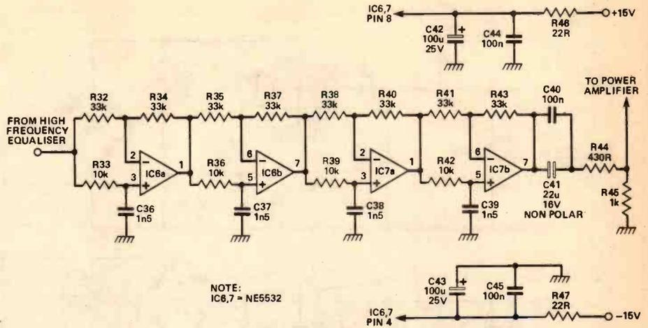
Fig. 11 Delay circuit.
