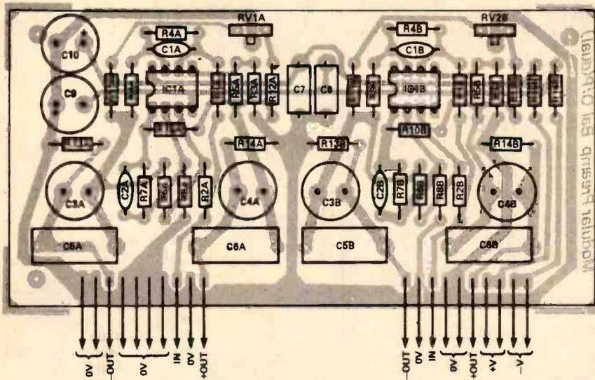
Fig. 2 Overlay of the PCB for the balanced output driver — this is a stereo board, so only one is required, but note the components that you have to obtain two of.
