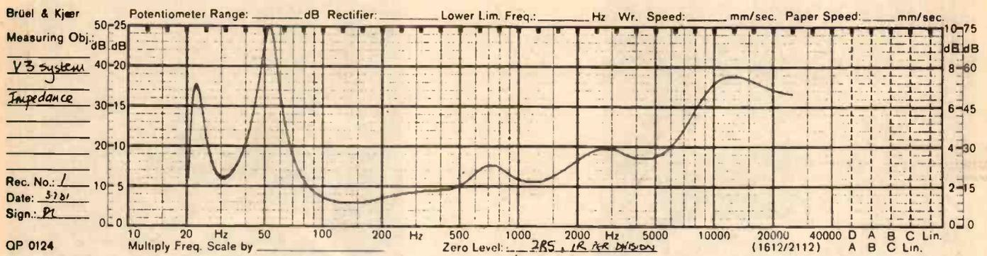
Fig. 1 Impedance curve for the V3 Loudspeaker.
