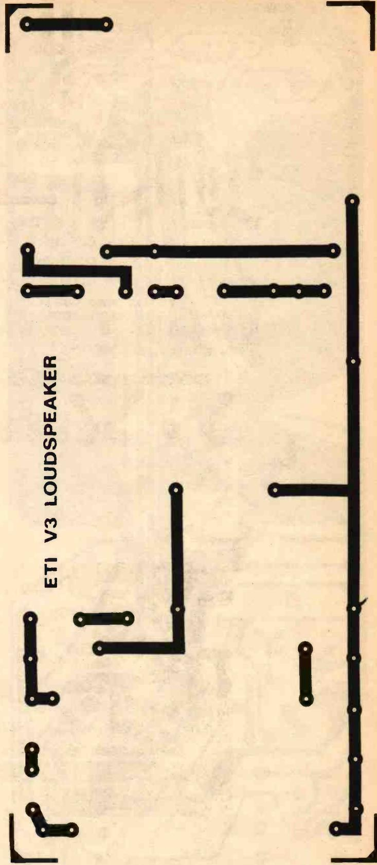
Above: the V3 loudspeaker system crossover PCB.
