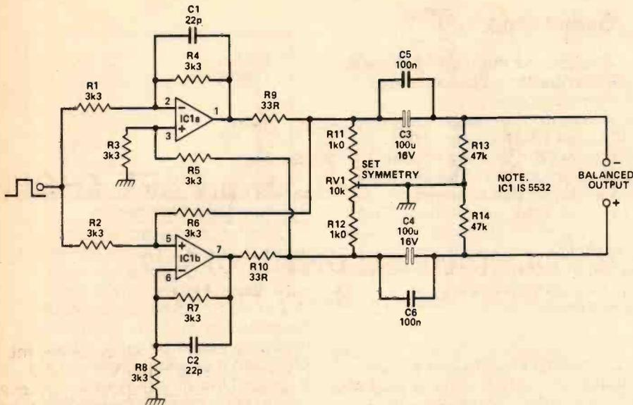
Fig. 6 Circuit diagram of the balanced output stage.
