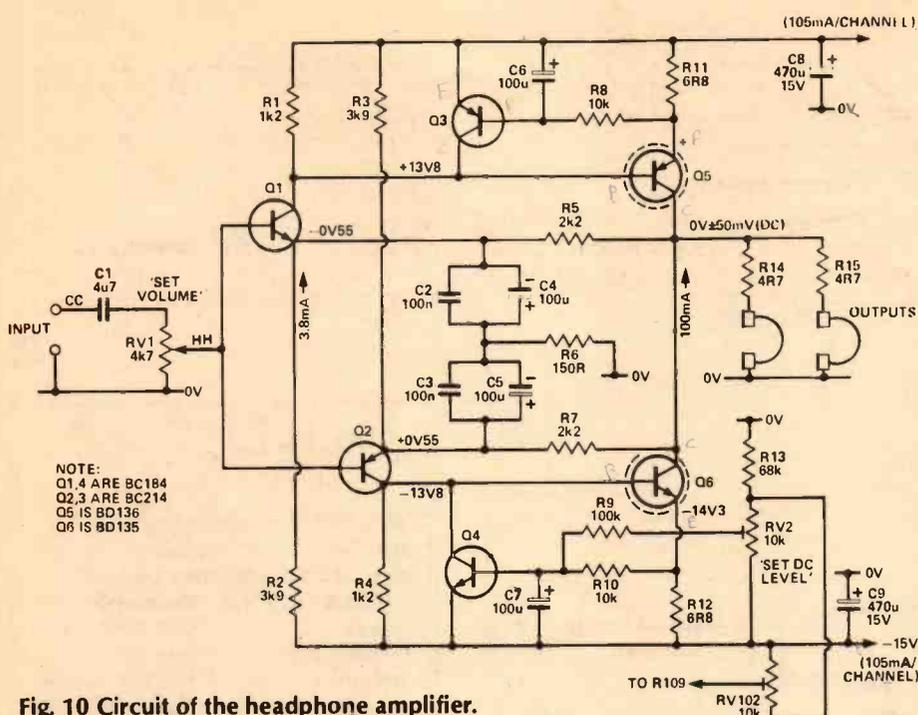
Fig. 10 Circuit of the headphone amplifier.
