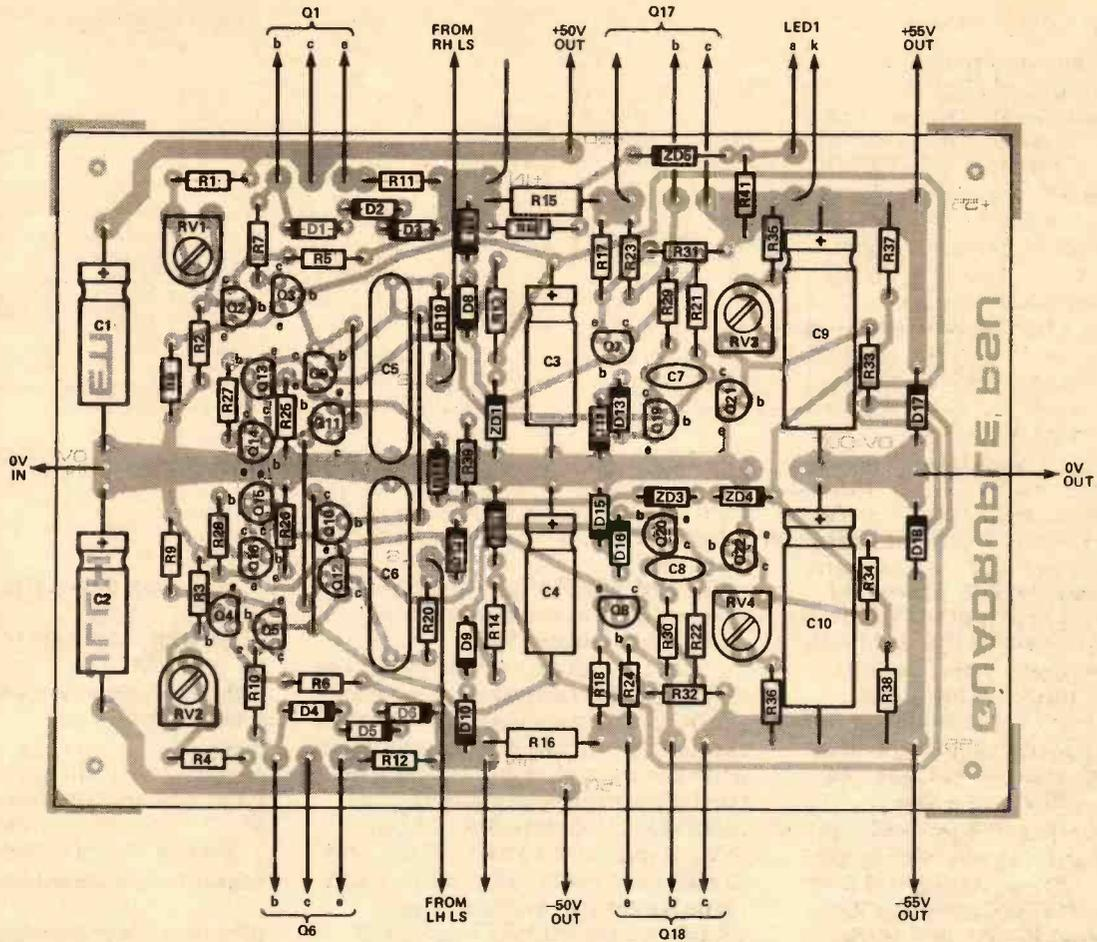
Fig. 9 Overlay diagram for the PSU.
