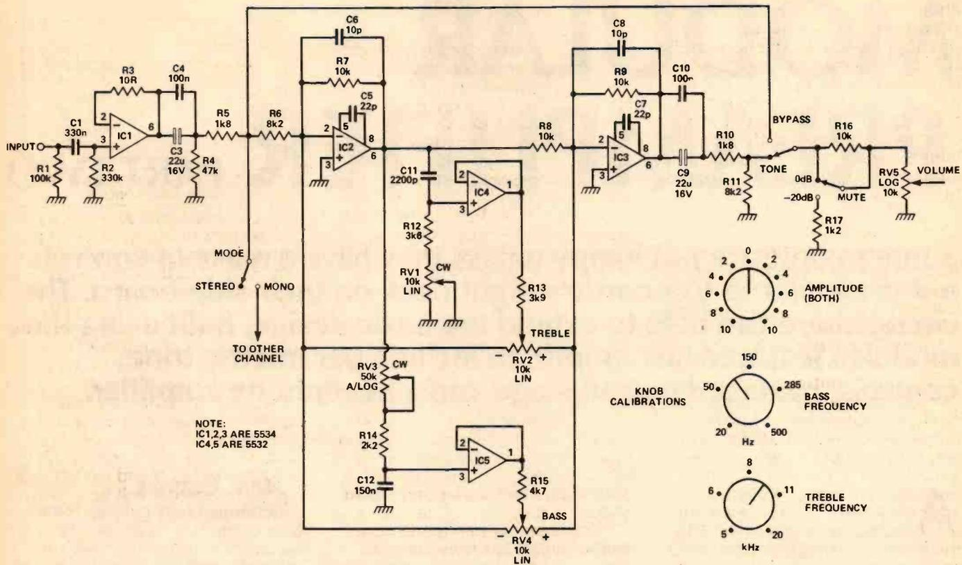
Fig. 2 Circuit diagram of the tone control module.
