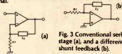
Fig. 3 Conventional series feedback equalisation stage (a), and a different configuration using shunt feedback (b).
