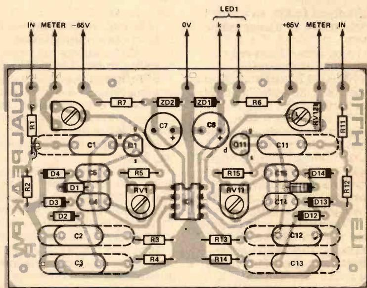
Fig. 14 Overlay diagram for the power meter.
