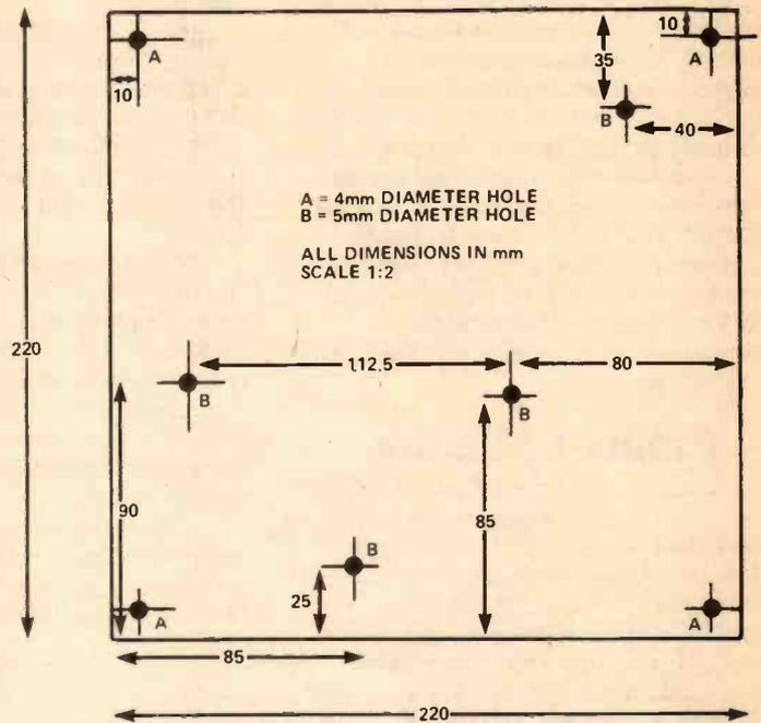
Fig. 5 This diagram shows the drilling positions for the choke and mounting screwholes on the crossover panel.
