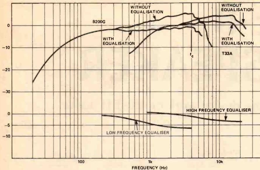
Fig. 8 Free-field response of the drive units.
