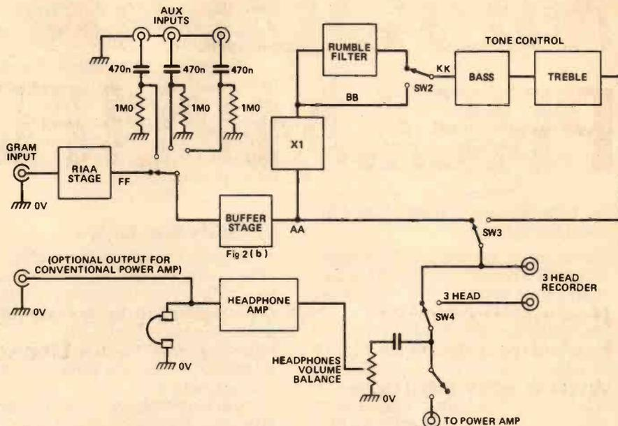
3 Alternative lay-out of preamp using discrete component buffer stage.
