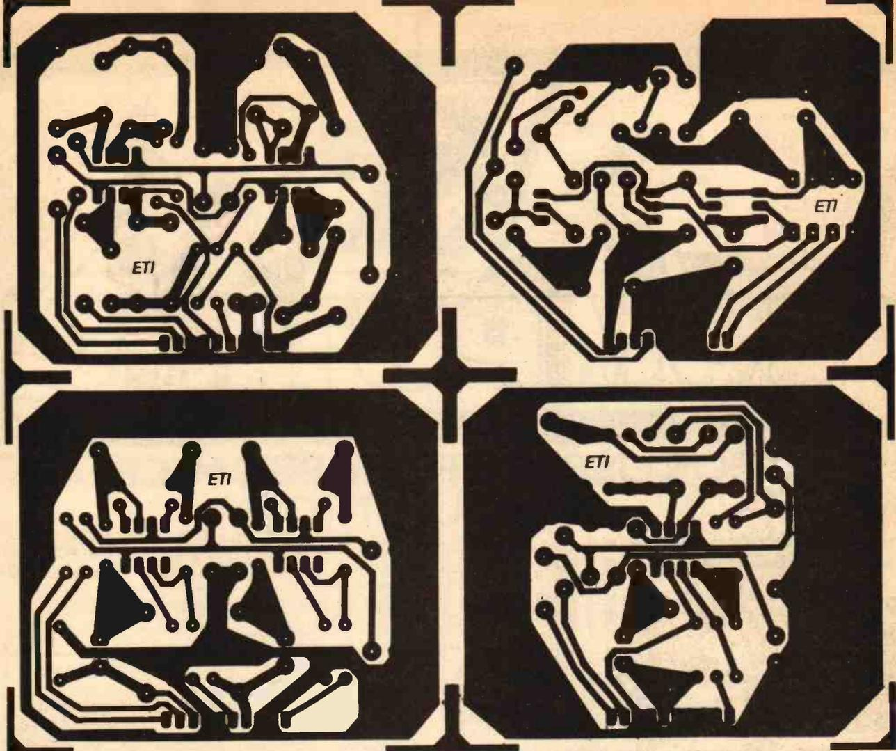
Above: the four plug-in modules for the Active 8 loudspeaker.
