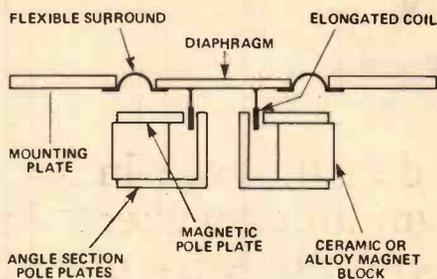
Fig. 2 Horizontal cross-section through the Musician drive unit.
