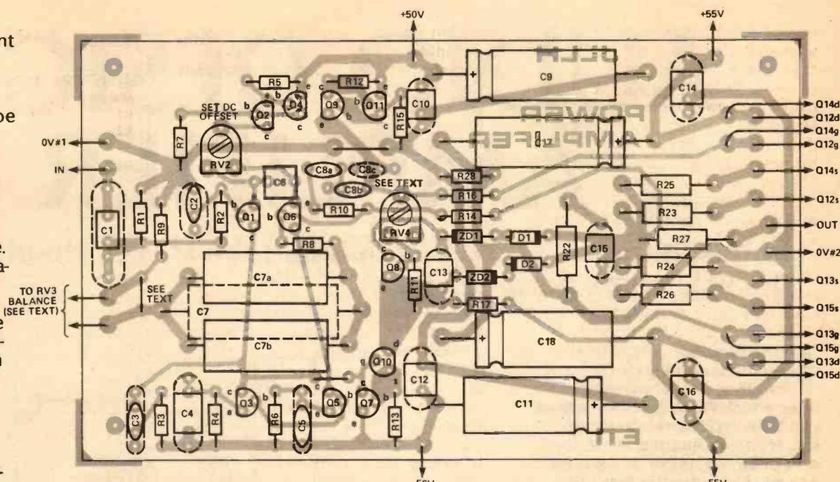
Fig. 7 The recommended PCB layout. Please note that the 'c' and 'e' labels on Q9 are reversed. The underlying PCB pattern is missing the link between the cathode of D1 and R16, RV4 wiper etc. This has been corrected on the foil pattern reproduced elsewhere in this issue, and on the board supplied by our PCB Service.
