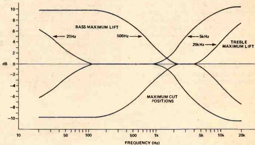
Fig. 3 Response curves for the tone control module.
