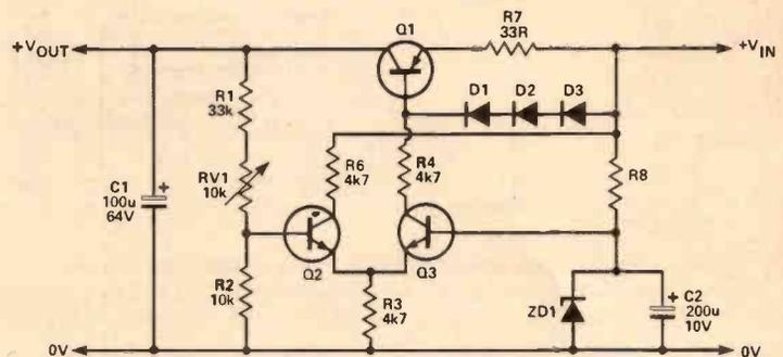
Fig. 1 Low-current stabilised PSU.
