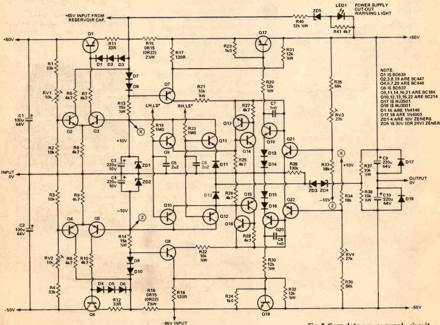
Fig. 5 Complete power supply circuit.
