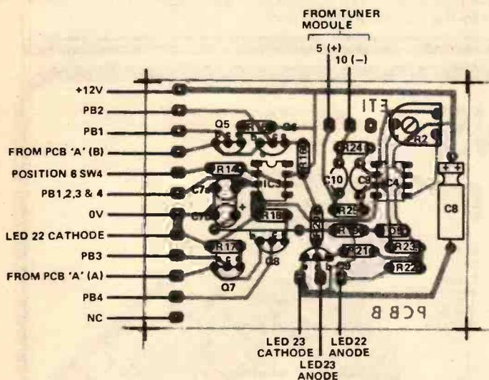
Fig.10 Component overlay of the auto search-lock network.
