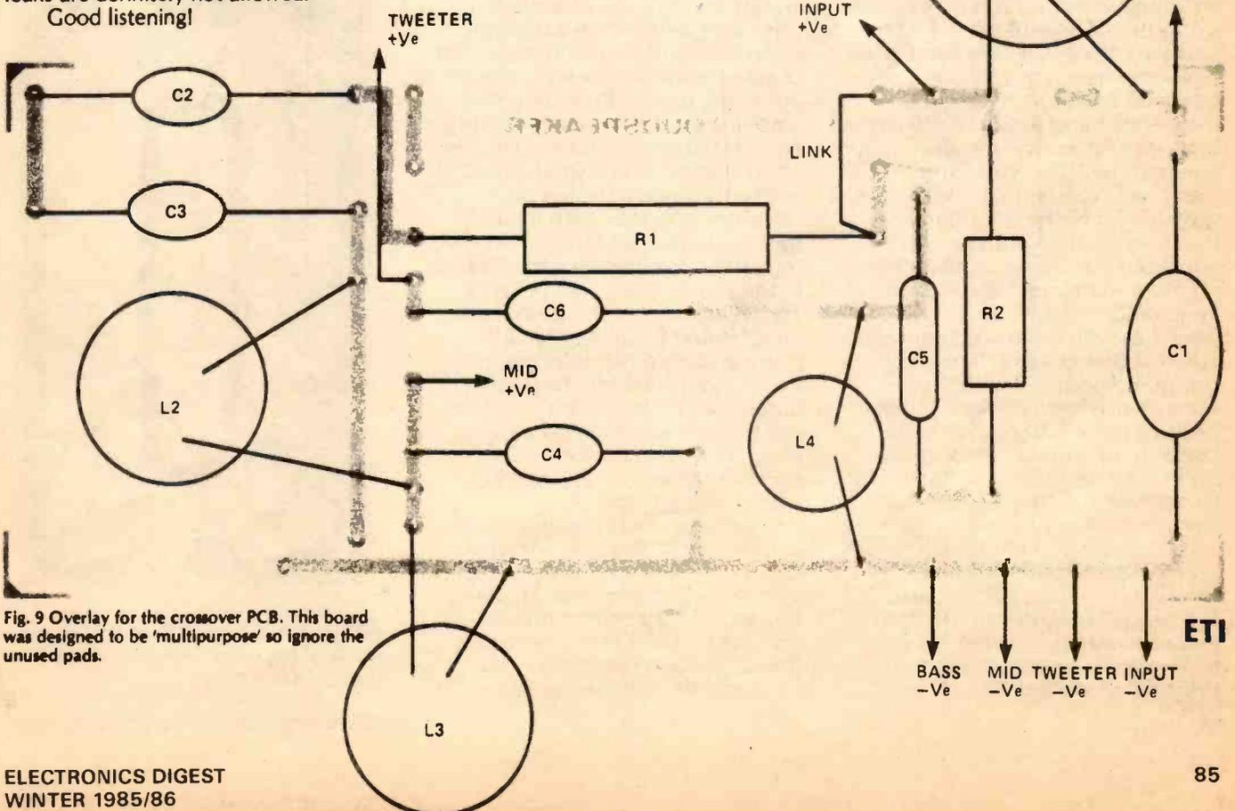
Fig. 9 Overlay for the crossover PCB. This board was designed to be 'multipurpose' so ignore the unused pads.
