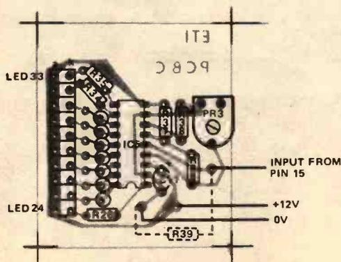
Fig.11 Component overlay of the signal strength meter.
