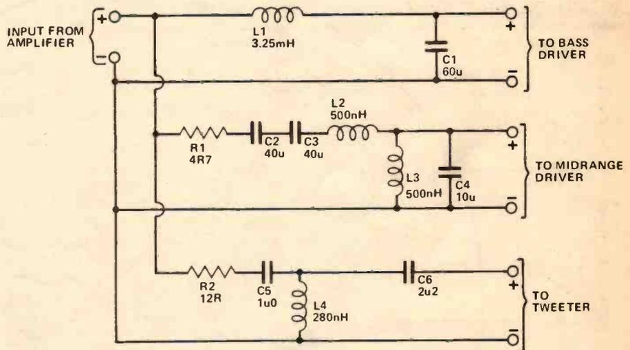
Fig. 6 Circuit diagram of the crossover.
