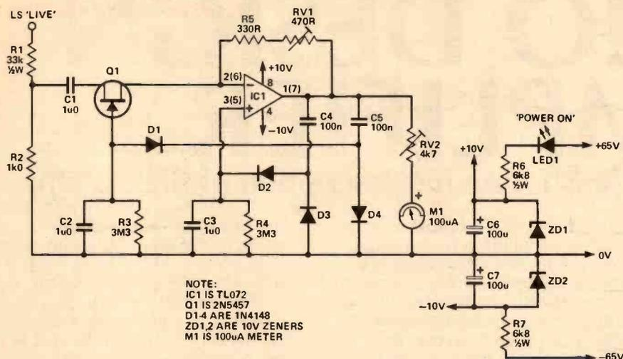
Fig. 13 Peak-reading linear scale power meter (8 ohms load).
