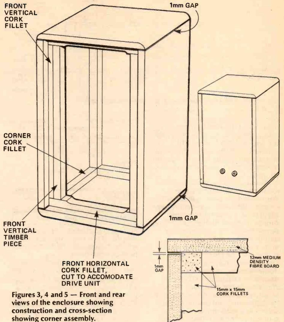
Figures 3, 4 and 5 — Front and rear views of the enclosure showing construction and cross-section showing corner assembly.
