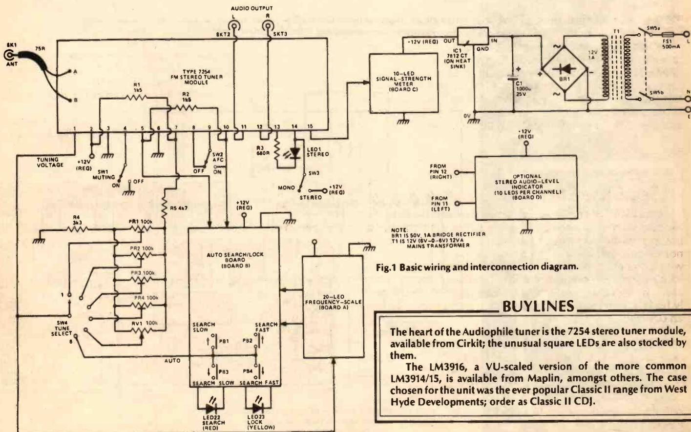
Fig. 1 Basic wiring and interconnection diagram.
