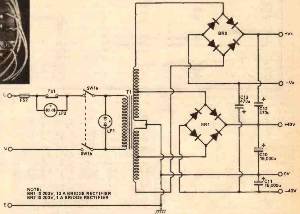
Fig. 4 The PSU circuit used to drive the power amps.
