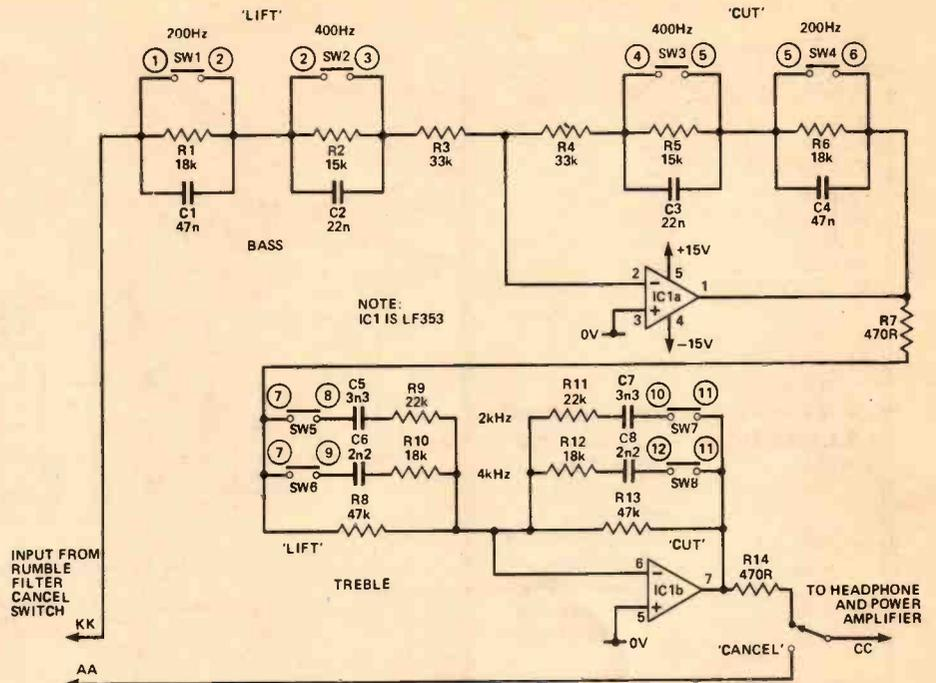
Fig. 5 Circuit diagram of the tone stage.
