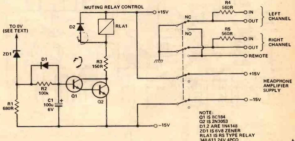
Fig. 7 Circuit diagram of the muting relay control.
