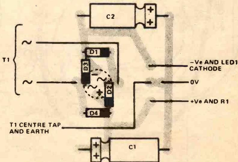
Fig. 1 The long-awaited preamp power supply overlay (and Parts List at top right). Provision has been made on the board for either four diodes or a small bridge rectifier, as shown.
