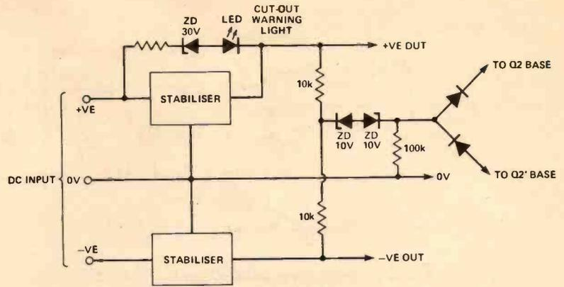
Fig. 4 Method of making both power supplies cut out simultaneously.
