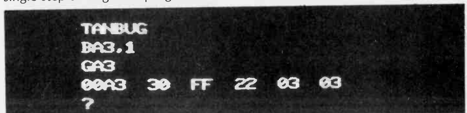
Fig. 2 Setting the first breakpoint at the start address and running the program gives this register printout.
