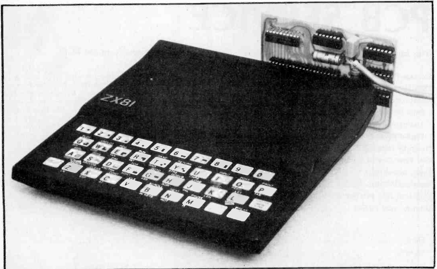
The ZX81 music and sound effects board, like most other ZX peripherals, plugs directly into the computer.
