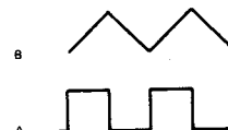
Fig. 11. (above) By making a loop out of a 7555, an inverter and an integrator, a triangle/squarewave oscillator is produced. To operate well at high frequencies (up to 40 kHz) a CMOS inverter should be used to replace the transistor inverter. The op-amp provides a low impedance triangle output, the frequency of which may be controlled with the 1M log pot.
