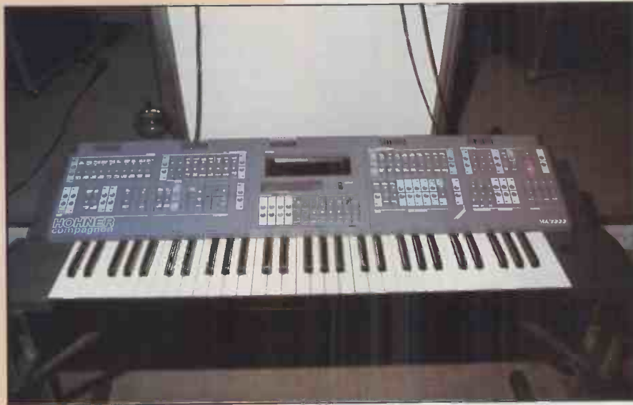
Astonishing Hohner Compagnon is designed to combine home organ ease of use with synthesiser versatility, was one of many 'modern' instruments from revitalised organ industry
