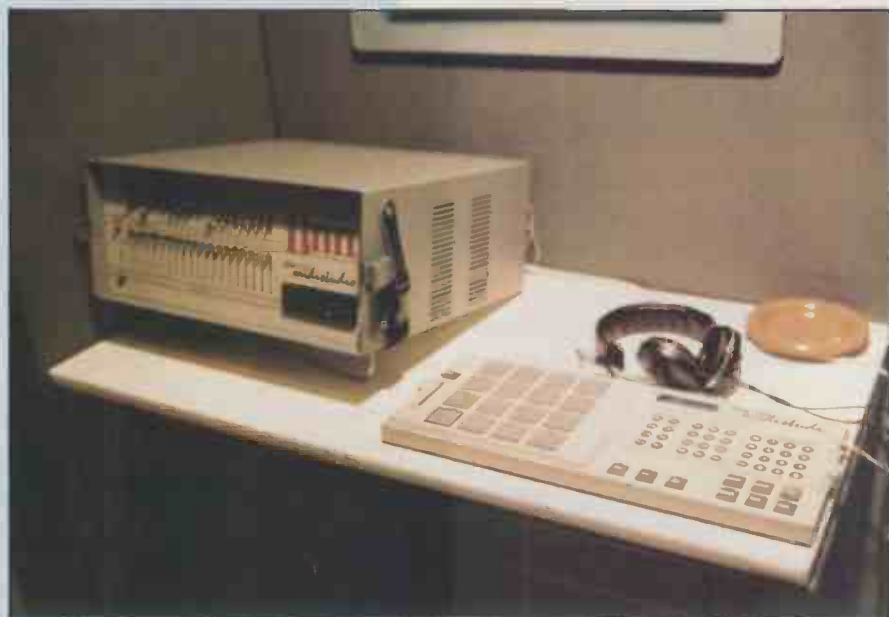
Attractive Linn MIDistudio is no more than repackaged Linn 9000, features 'lap pad' for remote programming in control rooms away from main unit, but costs no less than original machine
