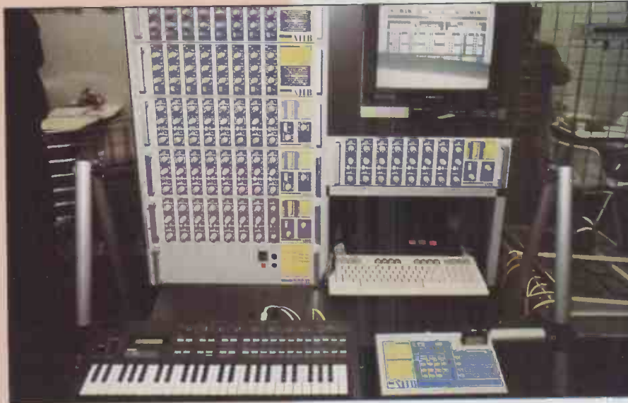
AHB Keymix system is sophisticated MIDI-based keyboard mixer network, made up of modules you can buy individually; remote control unit is prototype, other devices are available now
