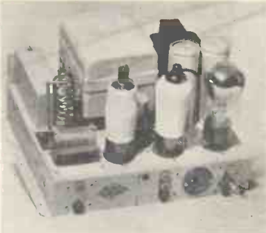
The chassis of the Union Radio superhet short wave converter, which has a self-contained power pack and is for A.C. mains operation.
