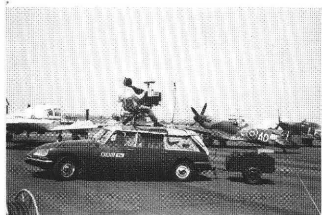
Fig. 2 Citroen Safari unit with camera mounted and towing its generator
