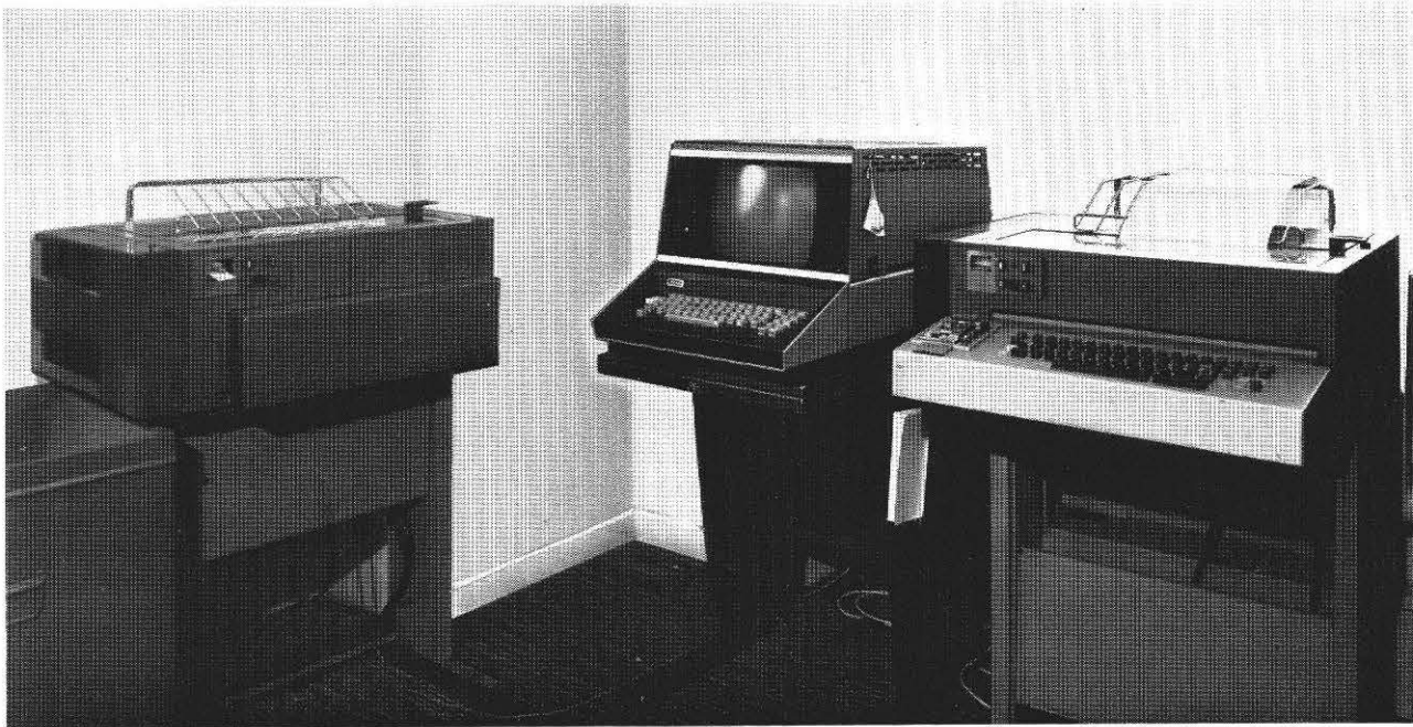
Fig. 4 Visual display unit flanked by 8-unit Olivetti reject and refile teleprinters on the left and right respectively
