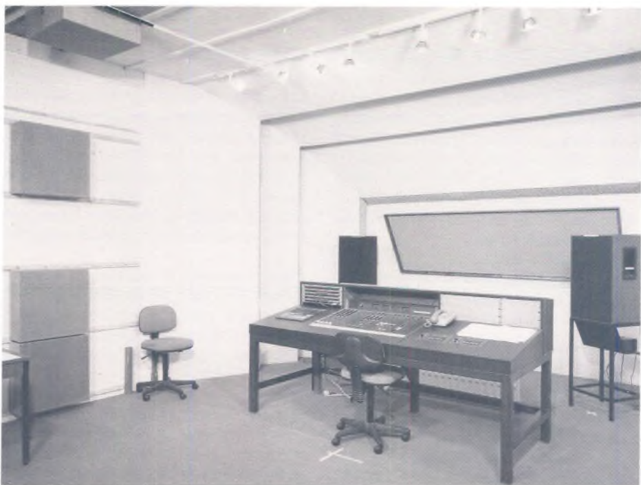
The acoustic test room at Kingswood Warren with an experimental reflection-free zone.
