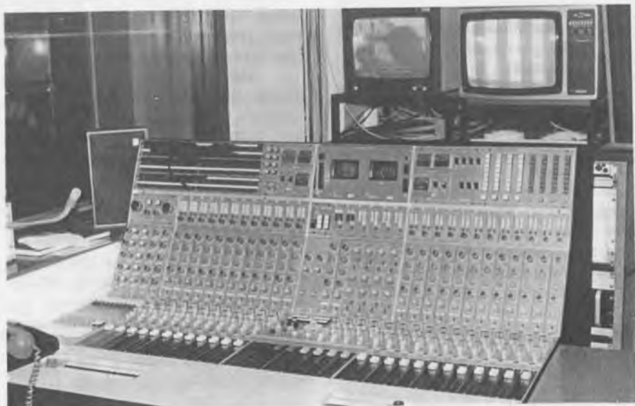
The Neve 24 channel sound mixing desk in the sound control room at the Greenwood Theatre.
