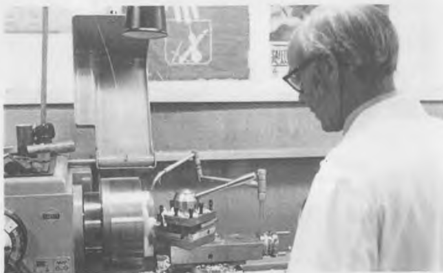
Jim Richardson turning P.T.F.E. aerial parts in the mechanical workshops
