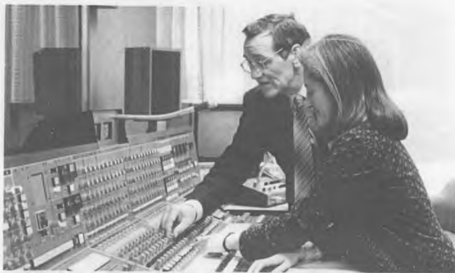
Sue Wilson, a Studio Manager, is shown the channel routing on the new Mark IV desk by Roy Spratley, SCPD.
