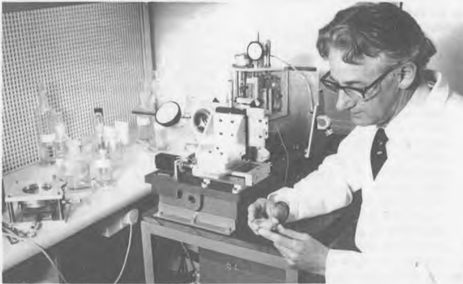
The photo-fabrication facilities and stepping camera used for experimental Surface Acoustic Wave devices at Kingswood Warren.
