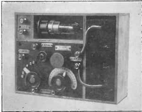
Fig. 41.—Photograph of Portable Single-valve Receiver.
