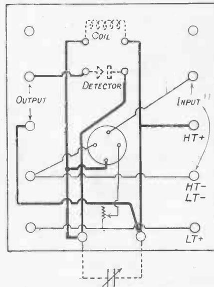
Fig. 84.—Wiring Diagram of H.F. and Detector Panel.
