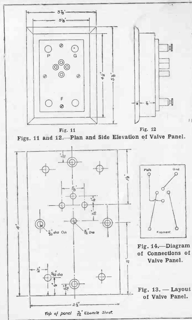
Fig. 11 and 12.—Plan and Side Elevation of Valve Panel.
