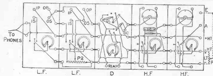
Fig. 113.—Wiring Diagram of Improved Set.
