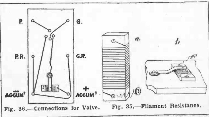
Fig. 36.—Connections for Valve.
