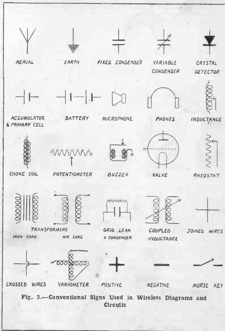
Fig. 3.—Conventional Signs Used in Wireless Diagrams and Circuits
