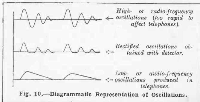
Fig. 10.—Diagrammatic Representation of Oscillations.
