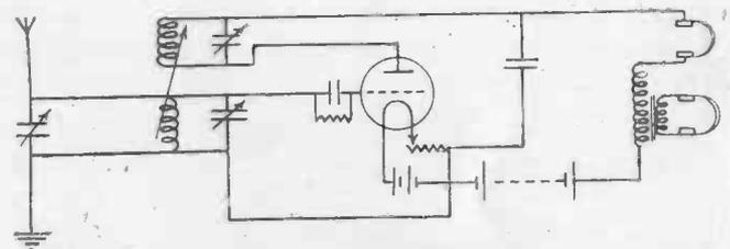
Fig. 53.—Two-coil Circuit.
