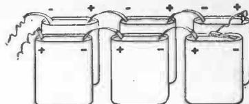
Fig. 39.—Method of Assembling H.T. Battery.
