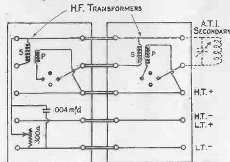
Fig. 107.—Potentiometer Connections of H.F. Transformer Panels.
