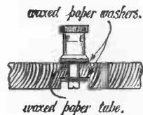
Fig. 34.—Insulation of Terminals.
