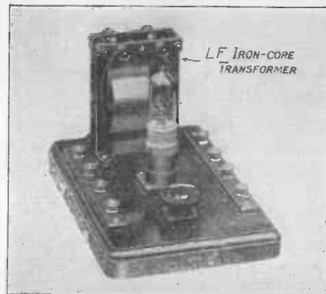
Fig. 89.—Photograph of Low-frequency Panel with Iron-core Transformer.
