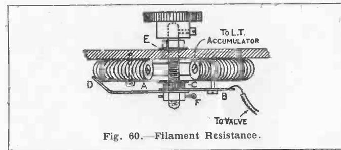
Now take about 3 yd. No. 21 s.w.g. "Chronic" resistance wire and wind it tightly round a lead pencil with the spirals touching. When removed from the pencil the spirals will keep their shape and the coil can be fixed to the ebonite disc in the place allotted to it. The turns of wire should not touch then.
