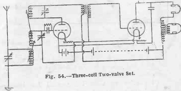
Fig. 54.—Three-coil Two-valve Set.
