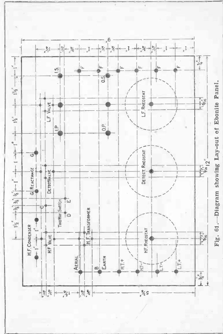
Fig. 61.—Diagram showing Lay-out of Ebonite Panel.
