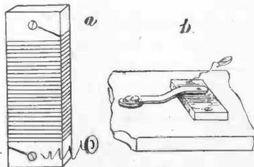
Fig. 35.—Filament Resistance.
