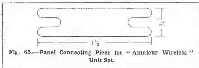
Fig. 65.—Panel Connecting Piece for "Amateur Wireless" Unit Set.
