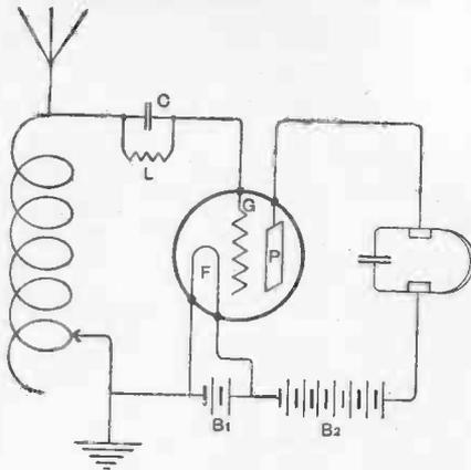
Fig. 9.—Valve as Detector and Low-frequency Amplifier Combined.
