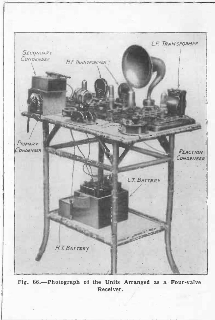
Fig. 66.—Photograph of the Units Arranged as a Four-valve Receiver.
