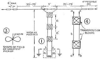
Fig. 3.—Shape of field. Fig. 4.— Fig. 1.—Horizontal doublet. Transposition blocks
