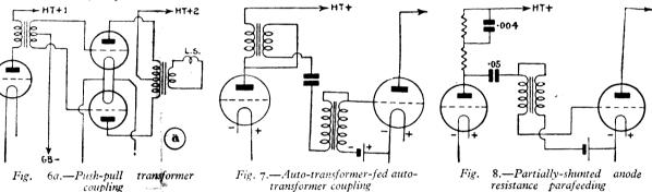
a coil winding offers an impedance to a transient signal, while the pure non-inductive resistance offers very little.
