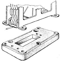
Low-loss Steatite base for short-wave variable condenser
