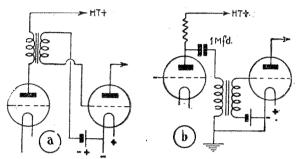
Fig. 1.—Transformer coupling, fed (b) direct (a) and parallel-
