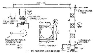
Fig. 2.—Inverted L aerial. Fig. 5.—Shape of field. Fig. 6.— Transposition block. Fig. 7.—Coupling coils
