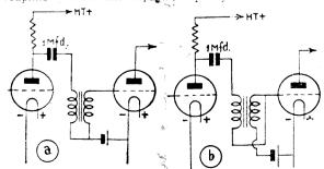
Figs. 5a and b.—Parallel-fed auto-transformer coupling
