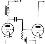
Fig. Choke-capacity 3. coupling
