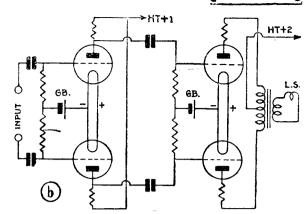
Fig. 6b.—Push-pull resistance coupling
