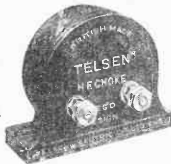
Telsan H.F. Chokes. Designed to cover the whole waveband range from 18 to 4,000 metres, extremely low self capacity, shrouded in genuine bakelite. Inductance. 150,000 microhenries; resistance. 400 ohms. Price 2/6 each.
