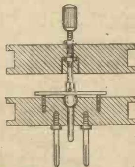
Simple Reaction Coupling Device.
