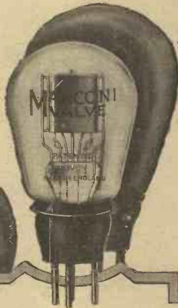
Type DE5. A dull emitter for L.F. amplification. Recommended as last valve of an amplifier using R5V or other valves running from 22/6 a 6-volt accumulator. Price 22/6
