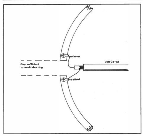
Fig 2: Detail at 'A' on Fig 1. Note: if the array is not erected in a roofspace, a separate/centre insulator will be necessary
