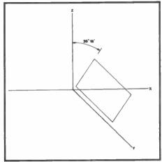
Fig 2: The AT crystal cut with relation to the crystal axes
