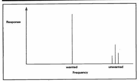
Fig 4: The responses of a crystal showing the unwanted modes
