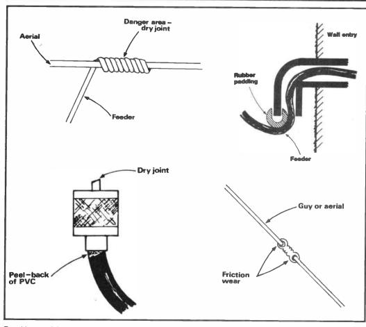
Repairing dry joints and friction wear
