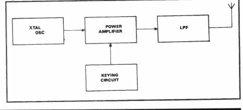
ers and have dozens of memories together with computer control etc. **Fig 1** is an example of a typically simple QRP transmitter.
