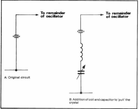
Fig 2: Modifying a crystal oscillator to be a VXO
