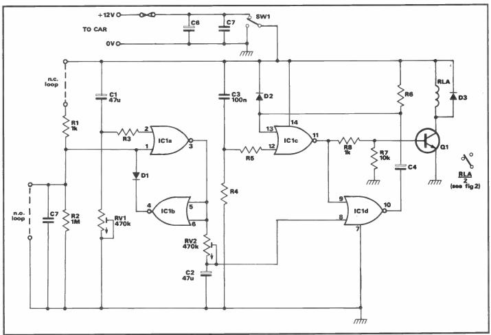
Fig 1: The alarm circuit layout
