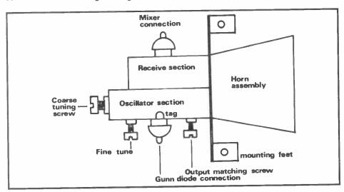
Fig 1: Microwave head assembly
