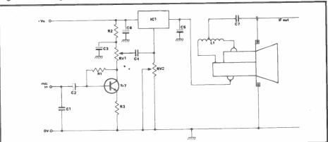
diode into the receiver you are going to use as the IF strip. This is done using the coil marked L1 in the circuit diagram, which gives an impedance step-down ratio of 4:1. This coil and its associated output capacitor should be mounted directly on the head and connected to the BC receiver via a short piece of thin 50 ohm coax cable.
