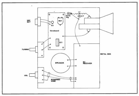
Fig 3: Layout of sub units in case
