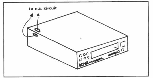
Fig 2c: Protecting a radio by drilling two small holes and passing insulating wire through them
