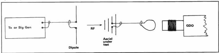
conjunction with a signal generator to test resonant circuits as shown in **Fig 3**. The techniques used are, however, similar to those used when just using the dip meter alone in an active way, so I'll leave discussion of this area of use until later in the series.
