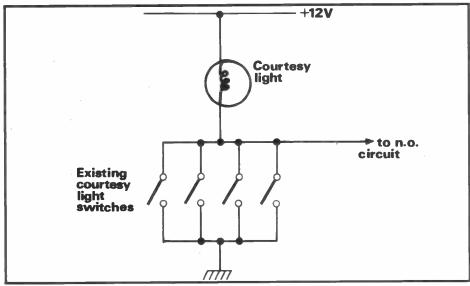
Fig 2b: Detecting the opening of the car door by using the existing courtesy light circuit
