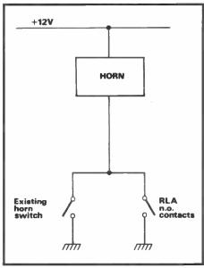
Fig 2a: Connecting the horn to the alarm circuit
