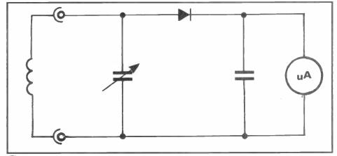
Fig 1: Typical absorption wavemeter
