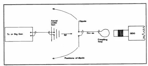
Fig 4: Checking directivity
