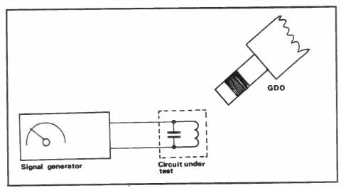
Fig 3: Using a signal generator
