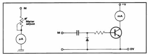
Fig 5b: Micrometer connection to the oscillator
