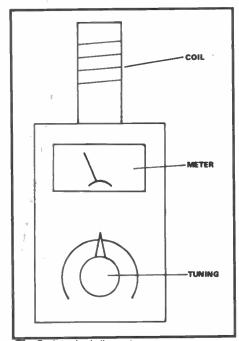
Fig 3: A typical dip meter
