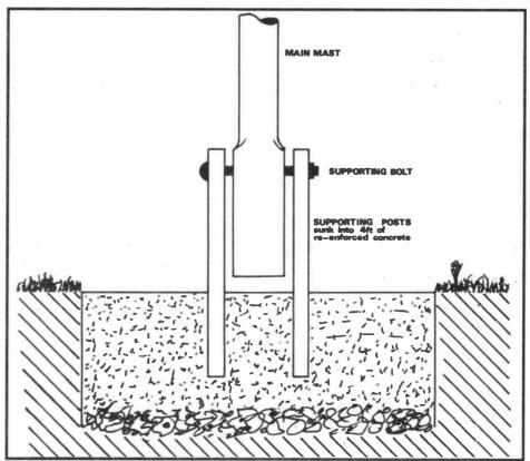
Fig 1: The two steel supports embedded in concrete
