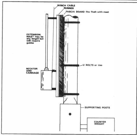
Fig 3: The carriage assembly
