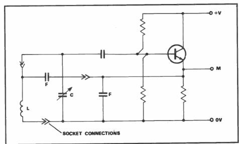
Flg 4a: First example of an oscillator circuit
