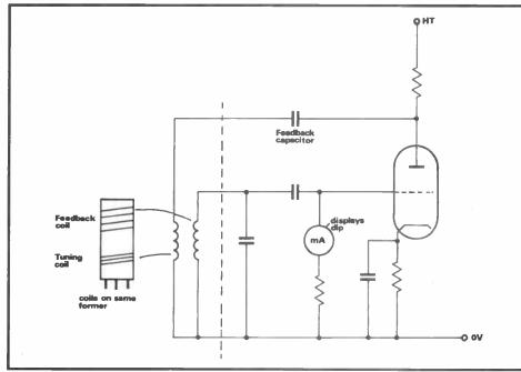
Fig 2: A valve oscillator with a grid circuit
