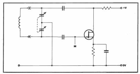
Fla 4c: Third example of an oscillator circuit
