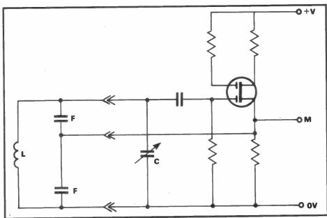
Fig 4b: Second example of an oscillator circuit
