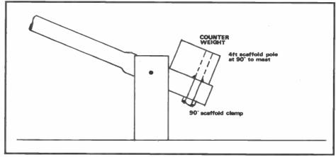
Fig 2: Showing how the mast pivots
