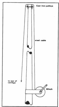
Fig 5: The pulley system
