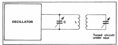
Fig 1: LC tuned oscillator
