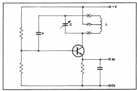
Flg 4d: Fourth example of an oscillator circuit
