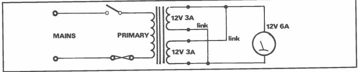
Fig 1: Parallel connected windings
