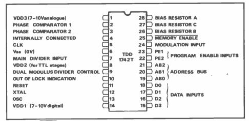
Fig 1: Pin out diagram for the TDD 1742T or Low Power Frequency Synthesiser (LOPSY) integrated circuit
