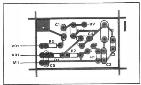
Fig 3: Component overlay
