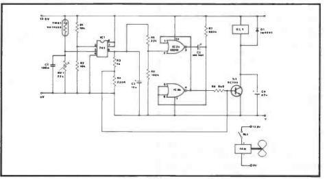
Fig 4: Circuit diagram of the temperature switch. TMS1 is on a remote board mounted on the heatsink of the PSU
