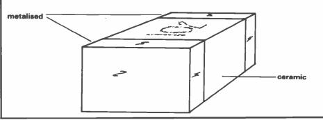
Fig 1: A chip capacitor
