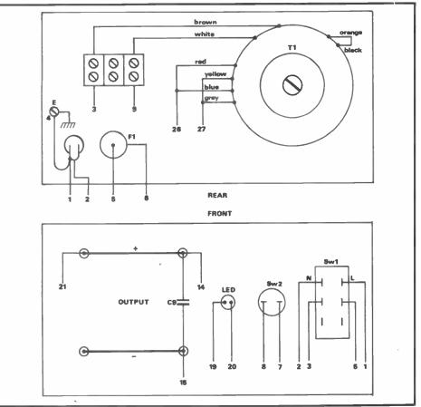
Fig 10: Front and back view of the case. The wiring has been numbered and can be checked with Table 1 below
