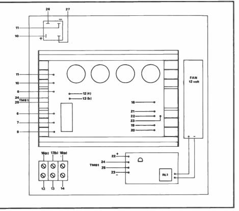
Fig 11: The base of the box. The main PCB is fitted over the heatsink to save space
