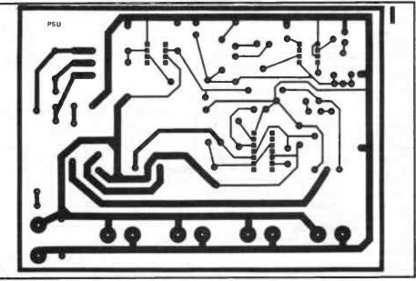
Fig 6: The foil pattern of the main PCB
