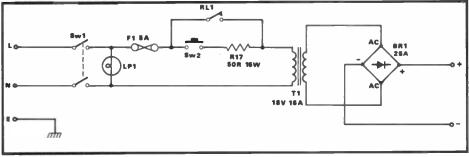
Fig 2: Circuit diagram of the first half of the power supply. T1 is rated at 13V 16.5 amps RMS and RL1 forms part of the protection circuits
