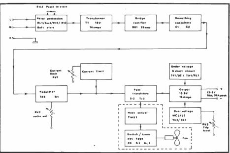
Fig 1: Block diagram of the power supply. The dotted area indicates the temperature switch and is not part of the main PCB
