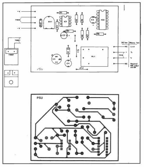
Fig 7: (top) component overlay of the temperature switch. Fig 8: Temperature switch PCB foil pattern
