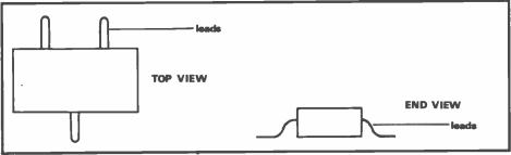
Fig 2: A surface mount transistor
