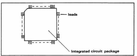
Fig 3: A typical surface mount IC
