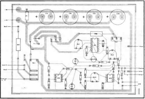
Fig 5: Component overlay of the main PCB. R13 and R17 are mounted off the board using 16swg tinned copper wire
