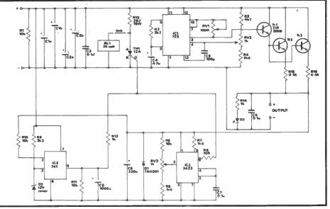
Fig 3: Circuit diagram of the main control board. Most of the components are mounted on a single PCB
