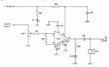
Fig 9 Component layout for the 8 pin LM380 audio amplifier
