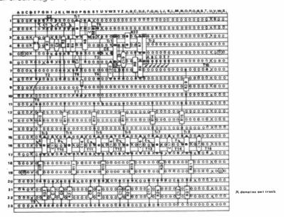
Fig 3 Component layout of master oscillator circuitry
