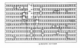
Fig 10 Component layout for the 14 pin LM380 audio amplifier
