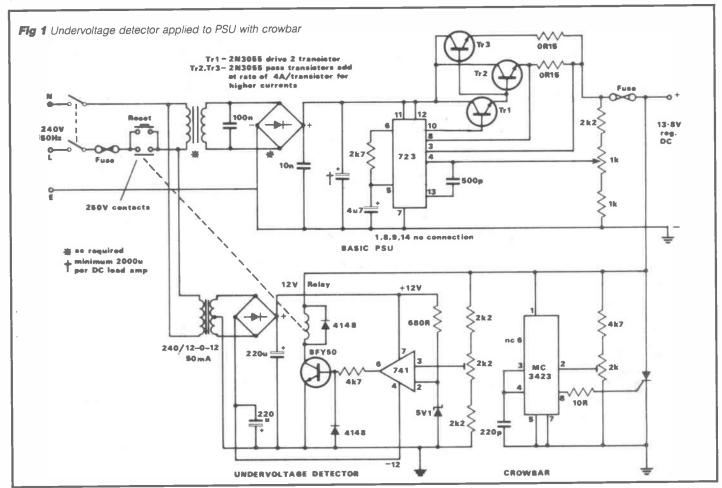
able, and in any case, a damaged thyristor invariably short circuits, thus failing safe. It must be borne in mind that the primary object is to prevent damage to an expensive transceiver, if necessary at the expense of PSU components, the cost of replacement of which would be no more than a few pounds. It is a case of keeping things in perspective! However, let's take a look at what I think is a worthwhile refinement to the PSU protective systems.
