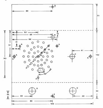
Fig 12 Dimensions of the back and bottom panels for head end amp case
