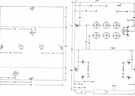
Fig 5 Dimensions of the front panel of the master oscillator box
