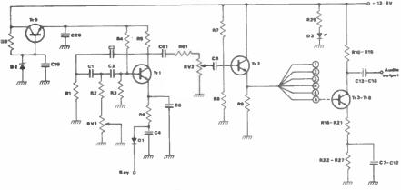
Fig 2 Full circuit diagram of master oscillator
