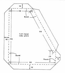
Fig 4 Dimensions of the two side panels
