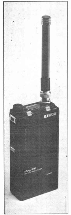
power switch. On the top of the rig is a BNC socket for the short rubber duck (111mm long) supplied with the rig. On the top panel is a miniature volume control with on/off switch, an absolutely tiny squelch control, and miniature lever switches which are spring loaded for changing memories up and down and for changing frequency in 1MHz, 100kHz and 12.5kHz steps. Each of these can be pushed or pulled lightly from a centre position to change a step.
