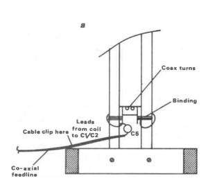
Fig 7 Simplified circuit configuration
