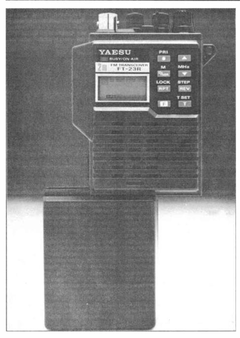
was about 10cm for an average voice, and if I spoke a lot closer the modulation went into limiting and the transmission became somewhat muffled, which is to be expected as the limiter is before the pre-emphasis.
