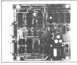
The SDS BOWMAN – The 68000 based single board computer for advanced high speed applications.
