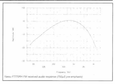
published plot shows that the transmitted response is within 6dB or so from 200Hz to 4kHz, and is thus appreciably wider than the receive response. I feel this is about right in practice for the UK market, although inappropriate for 12.5kHz chanelling. We noted only 1% THD at 4.5kHz deviation and this is excellent, the transmitted signal-tonoise ratio being very good.
