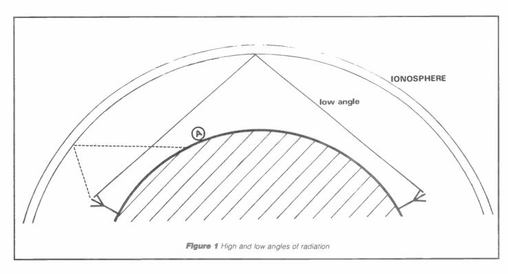
The vertical antenna offers the attraction of low angle radiation which is necessary if you intend working long distance stations (DX) on the amateur high frequency bands, 1.8 to 30MHz.
