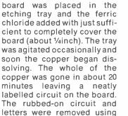
the resist remover. The next job was to drill the holes in the board with the bit provided in the kit which took about 15 minutes.
