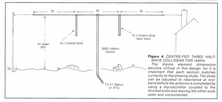
the antenna. The gain is of course in the two major lobes which lie at right angles to the wires. For the best results the antenna must be up at least 30 to 40 feet when it is designed for 14MHz, for if lower the radiation will tend to be at high angles and will be useless for DX working.
