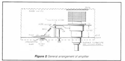
This wide range effectively compensates for variations in cavity size. It should be borne in mind, however, that resonance should not be obtained at either extreme of C4, otherwise retuning to a different frequency may not be very easy.
