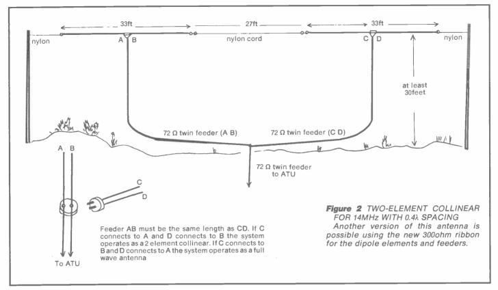
feed rules will apply; the feed line must drop away vertically from the top for at least a quarter wavelength on the design frequency and if possible it should not run below one of the 'legs' of the antenna. Imbalance will distort the radiation pattern which might then be slewed from the expected position which is at right angles to the wire. I have used several versions of this simple collinear and they have always given good if not outstanding performances.
