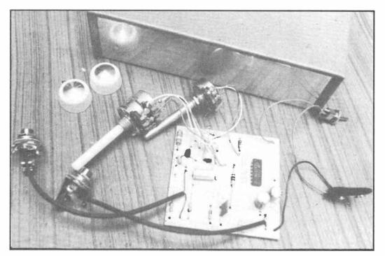
at the same temperature as the applied solder to give a good joint. The appearance of the joint should be shiny and only sufficient solder to make the joint secure should be used so concave 'shoulders' should be evident. Always trim off any surplus leads just about the joint to help prevent any chance of a short circuit. Also ensure that no solder has seeped into a gap between the copper tracks (bridging).
