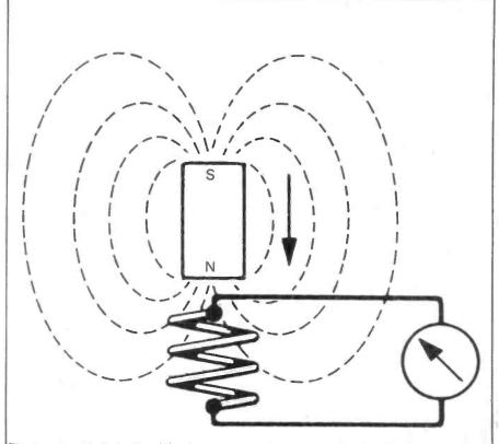
Electromagnetic induction (a) relative movement of magnet and coil induces a voltage in the coil; without this, there wouldn't be any wireless!
