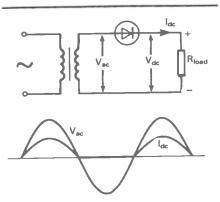
Half-wave rectifier and waveforms
