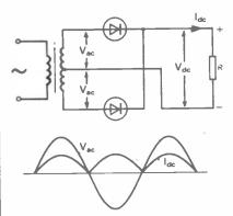
Full-wave rectifier and waveforms
