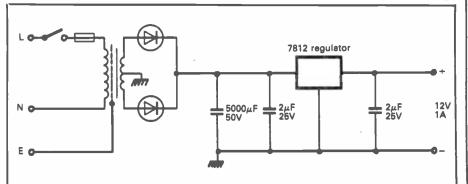
Practical power supply unit using ic regulator. The  $2\mu F$  capacitors should have short connections to the ic to prevent any unwanted oscillation.
