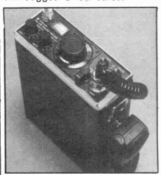
This is Trio's 144MHz hand portable (TR2300) which has 80 channels and around one watt outut on FM. Good audio sound.
