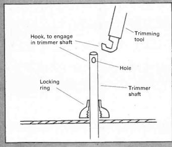
Above: This is a general guide to the control settings on AM, CW, SSB, and FM signals. There is, naturally, more information in the original manual - if you can obtain one. They are almost as valuable and rare as the equipment itself! Left: Details of the trimmer and the tool with which it can be adjusted. A well-kept AR88 should come supplied with two trimmer tools and an Allen key inside the cabinet.
