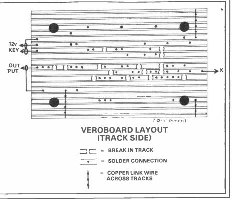
iron bit into the corner of the track and the wire and touch the opposite side of the wire/track junction with the solder so it is melted by the wire, not directly by the iron. The solder should flow smoothly to make a small joint – but check for bridges between adjacent tracks.
