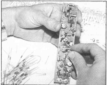
Fitting a tiny 82pF capacitor into the correct holes in the PCB.
