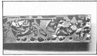
Close-up of the PA transistor soldered on to the PCB. Note the wide leads on the emitter of the transistor to keep the series inductance low.
