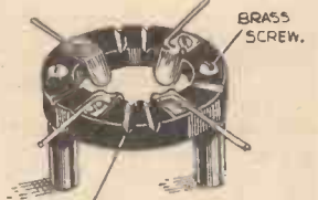
WEDGE SHAPED PCS. CUT OUT TO MINIMISE SURFACE LEAKAGE.
