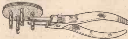
Fig. 1.—Showing simple method of compressing valve-holder socket to ensure good contact with valve pin.
