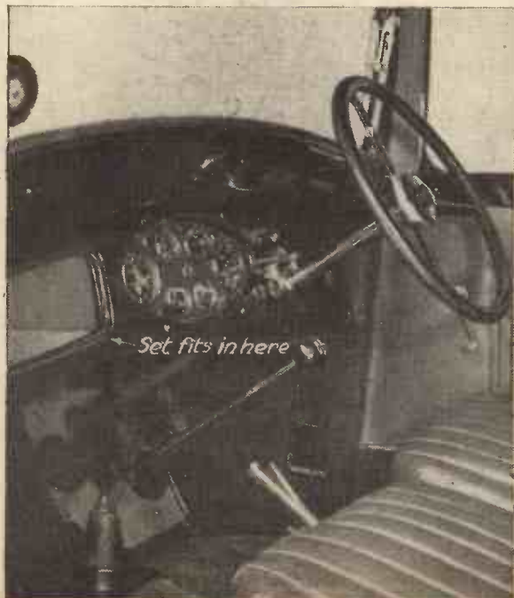
The receiver may be fitted into the glove-box of a car dashboard.
