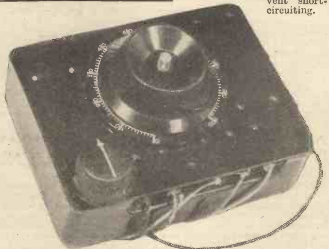
How the complete tuner appears in its case. The small spindle inside the tuning control is a trimmer.
