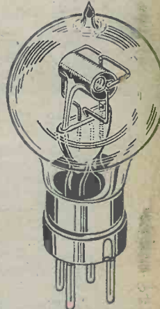
Fig. 5.—The well-known French "R" valve. This was extremely popular amongst amateurs immediately after the war, but its performance would be extremely poor compared with modern valves. It formed an ideal detector and was used in its thousands.
