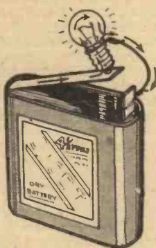
Fig. 1.—A simple example of the flow of a direct current is provided by this torch battery and bulb. The arrows show the path of the current.
