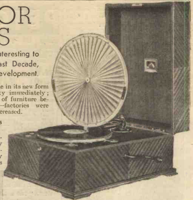
The Lumière diaphragm was applied to gramophones and loud-speakers in 1924 as a means of disseminating sound in place of a horn. In this instrument the vibrations from the record were transferred to the centre of the diaphragm by a system of bell-crank levers.
