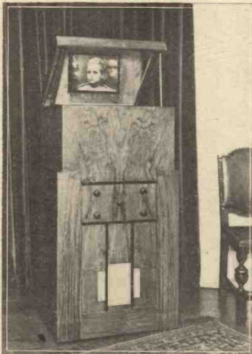
Fig. 3.—Employing a large cathode-ray tube mounted vertically so that the television images can be watched as mirror reflections, this modern instrument is ideal for home entertainment.
