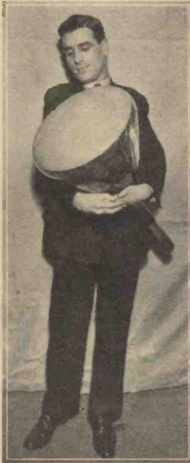
Fig. 2.—The largest Baird cathode-ray tube, giving a picture 12 in. square, being held by the youth whose face was the first to be televised in 1926.
