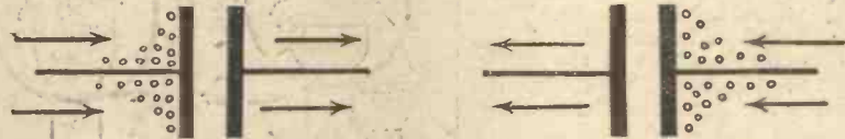
Figs. 12 and 13.—Diagrams illustrating the action of a condenser when subjected to an alternating current.
