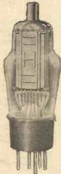
The Hivac valve shown above has only just been released—it is the mains-operated H.F. pentode.
