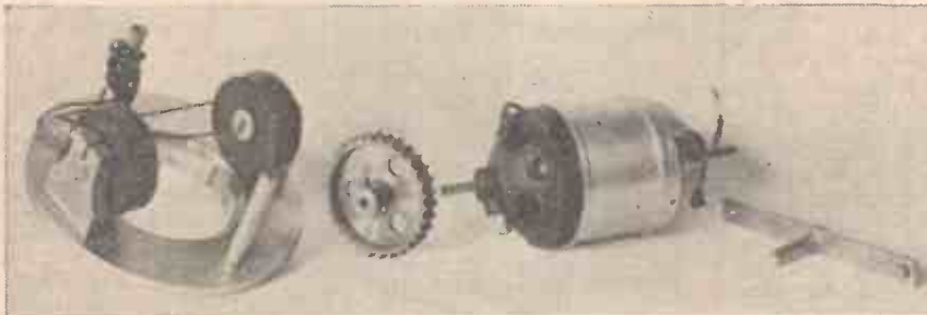
A small television motor with the synchronising mechanism partly dismantled to show the details.
