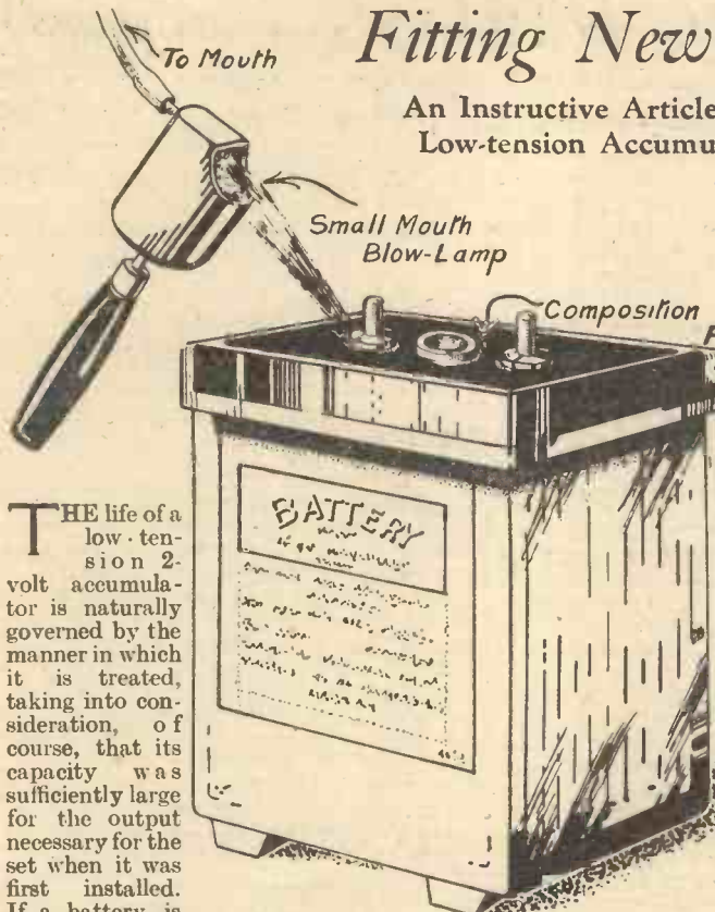
Fig. 3.—Using a small blow-lamp to finish off the pouring in of the composition.
