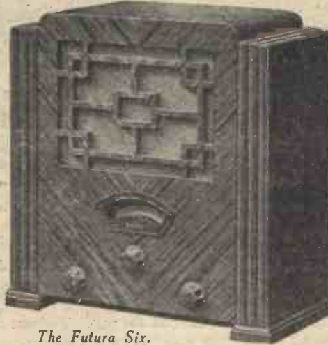
The Futura Six. An all-mains five-valve receiver.
