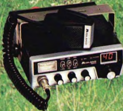
rtx mobile 5W AM 40 canali mod. 150 M
