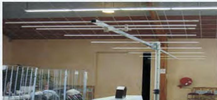
DX.S.R 902 Boom 25x2mm 30x2mm elements 10x1mm
