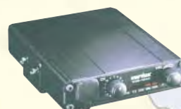
VXR-1000 Relais VHF/UHF mobile 16 canaux — 5 W
