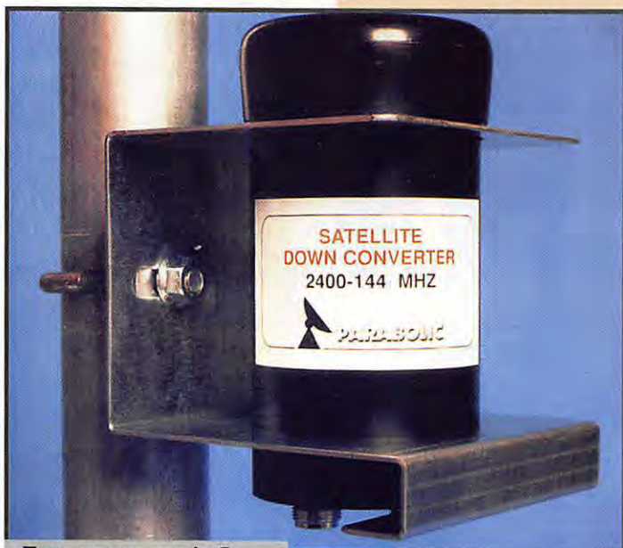
Transverter mode S 2400 → 144 MHz.
