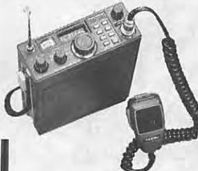
**YAESU - FT 203R.** Transceiver 144 MHz portable. FM. 3,5 W.
