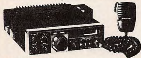
LS 102L - BELCOM : Transceiver 28 MHz Tous modes USB/LSB/CW/FM/AM - 10 W - affichage digital
