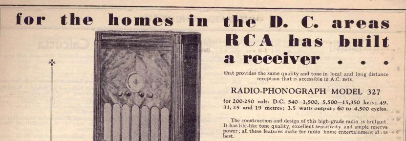
Model 327 is a six tube radio-phonograph combination for short and standard wave reception, operating from 220-volt direct current power supply. The electric phonograph has magnetic pick-up automatic tone compensation and inertis tone arm. The entire motor board spring mounted. The cabinet is of walnut veeneers, beautifully blended and the spring balanced is hinged so that it folds back from the centre. Record storage space is provided at the bottom.
