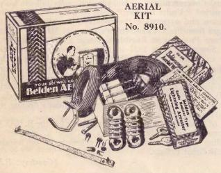
Contains 75 feet, 7"×26" Bare copper aerial. 25 feet, No. 18 stranded rubber Lead-in-wire. One Belden arrester 8896. One No. 8897 type C. Belden Ground clamp. One Belden 12" Lead-in strip No. 8890. Two Procelain insulators. Two Nailon-knobs. One Instruction sheet.
